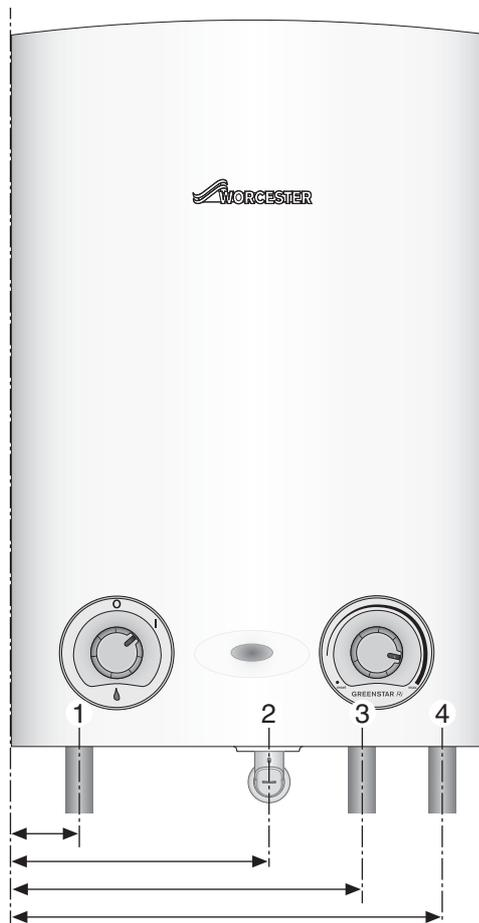
Fig. 19 Pipe work dimensions
