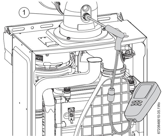
Fig. 62 Combustion test
