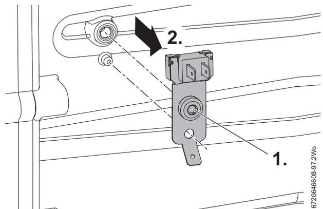
Fig. 73 Overheat sensor
