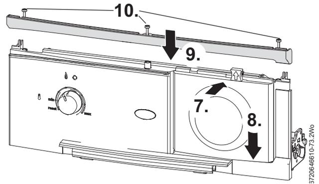
Fig. 40 Fitting the Programmer/Timer
