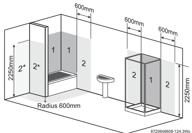
Fig. 12 Bathroom installations
