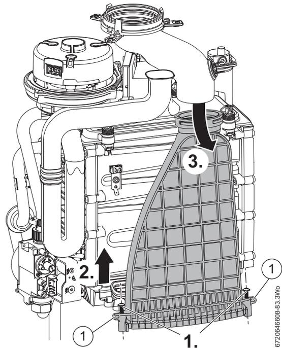
Fig. 79 Flueway removal
