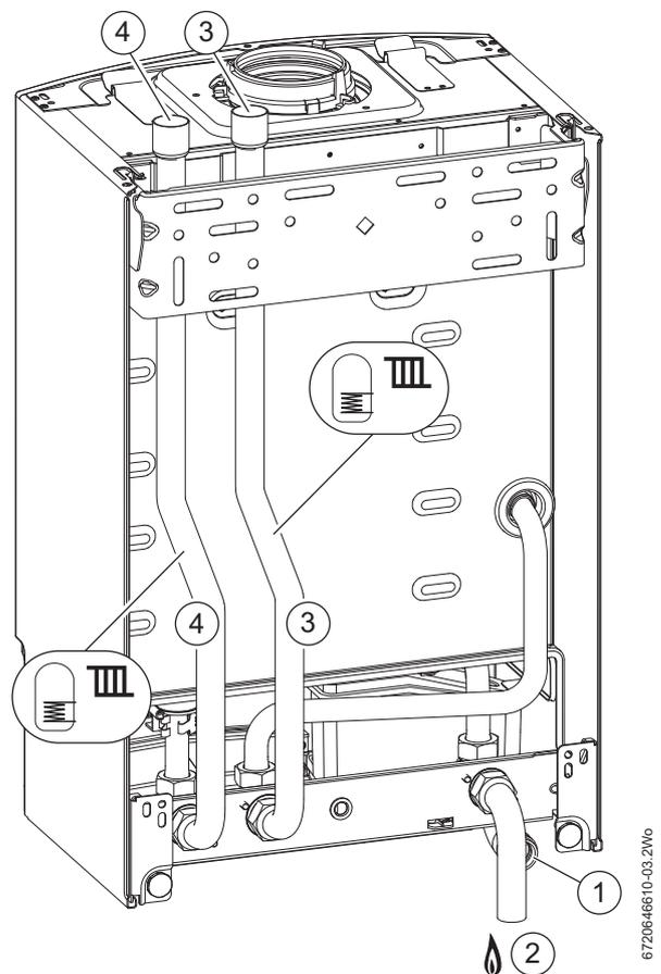
Fig. 27 Plumbing connections
