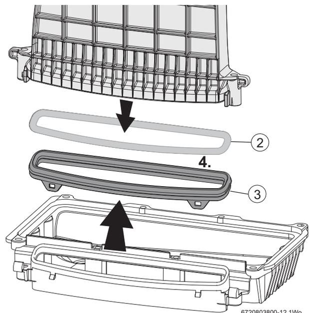
Fig. 80 Remove the existing seal
