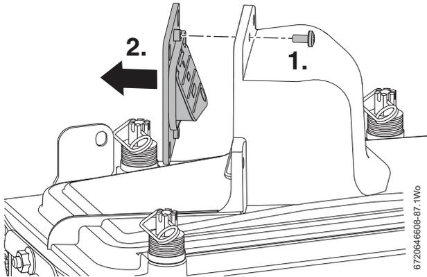
Fig. 86 Air/gas flap valve
