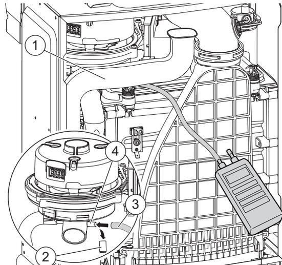
Fig. 59 Fan pressure test point
