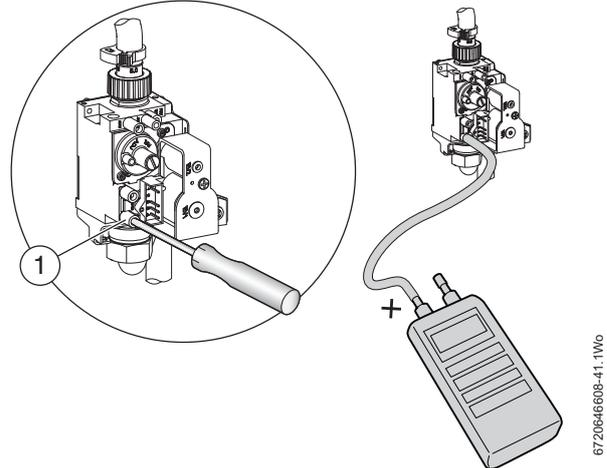
Fig. 48 Inlet pressure test point
