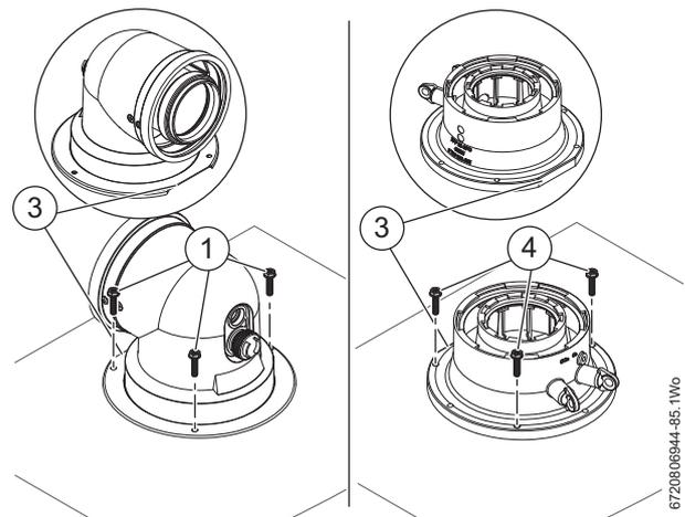
Fig. 34 Flue turret/adaptor connection
