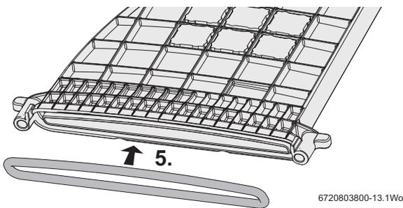
Fig. 82 Tubular style sump seal
