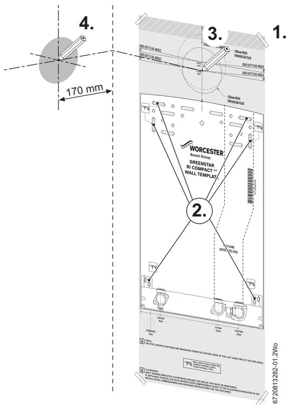
Fig. 22 Marking the flue position
