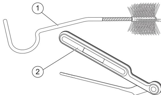
Fig. 65 Single-bladed cleaning tool and brush
