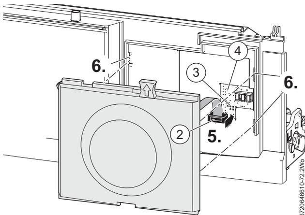
Fig. 39 Connecting the Programmer/Timer
