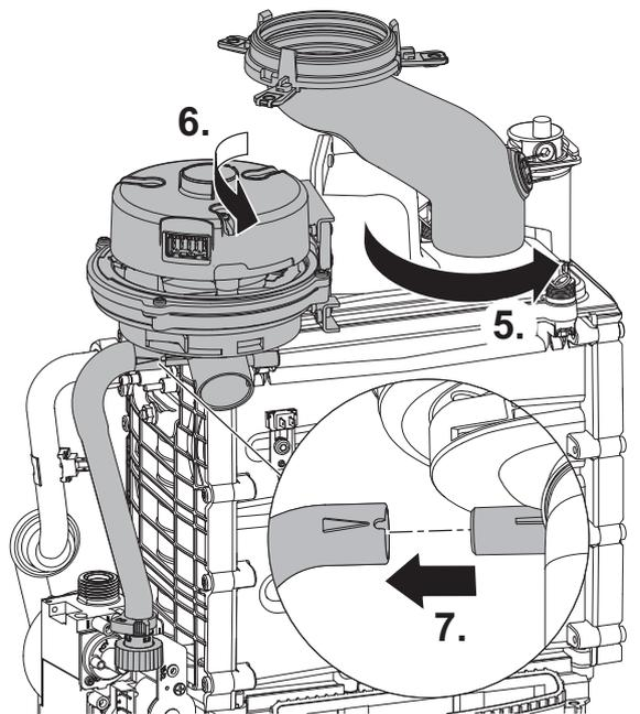
Fig. 85 Fan removal 2
