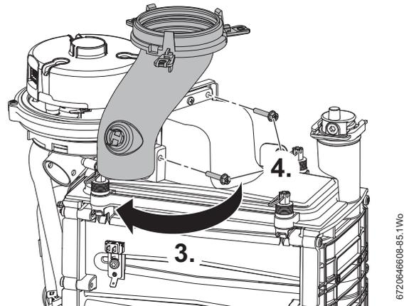
Fig. 84 Fan removal 1
