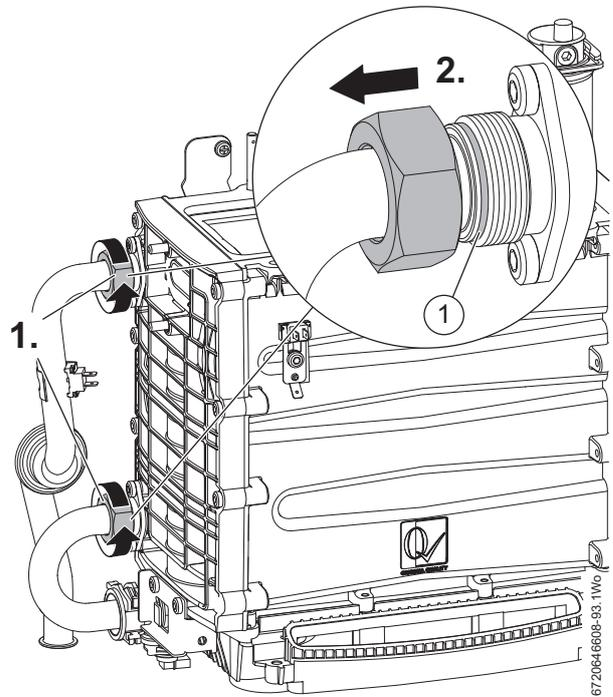
Fig. 92 Heat exchanger disconnection
