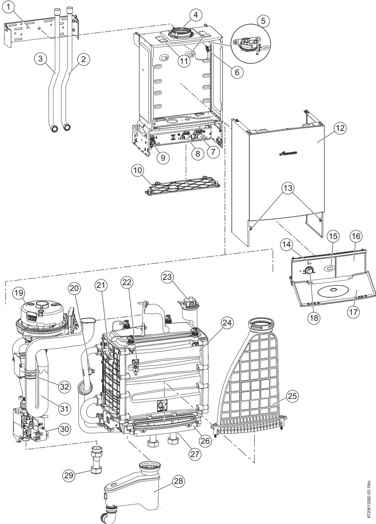
Fig. 2 Ri Compact ERP main boiler components
