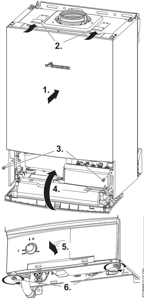
Fig. 52 Fitting case
