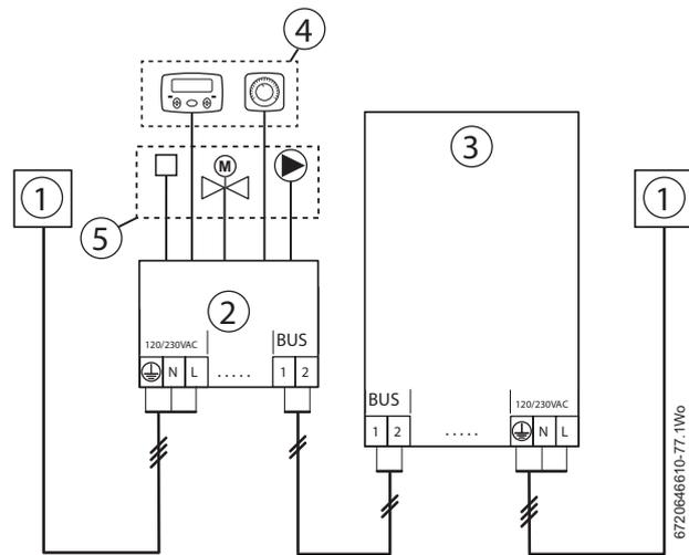
Fig. 42 Example Greenstar wiring centre
