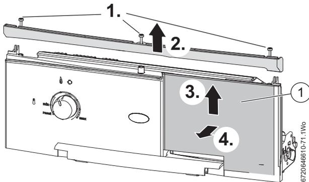
Fig. 38 Removing the blanking plate
