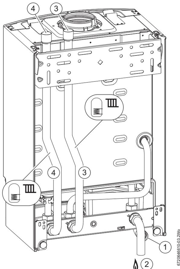
Fig. 14 Plumbing manifold
