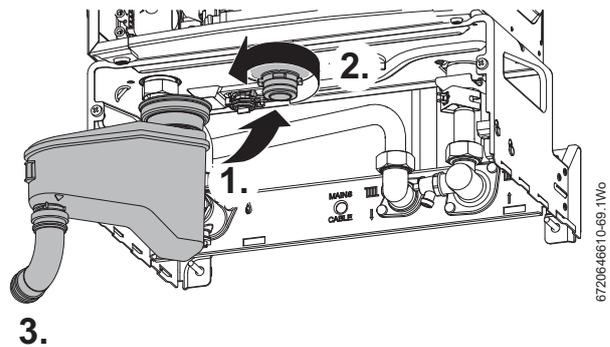
Fig. 64 Fitting siphon
