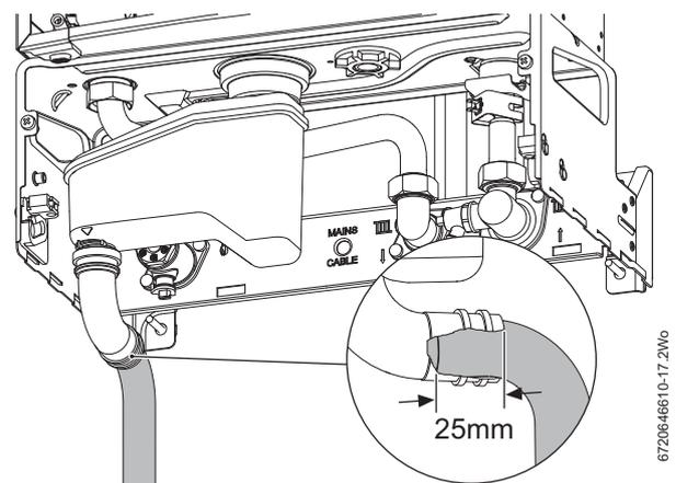
Fig. 44 Condensate connection
