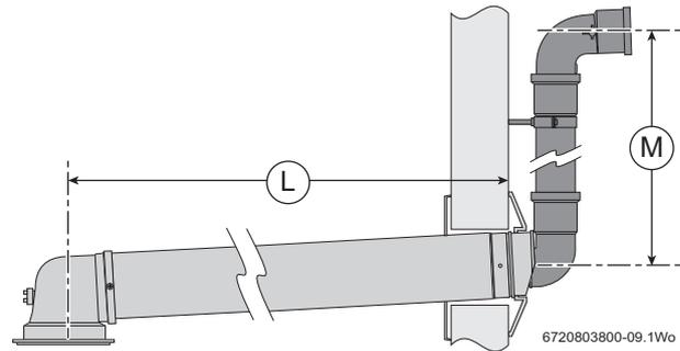
Fig. 18 Effective lengths L and M
