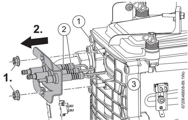
Fig. 88 Electrode assembly
