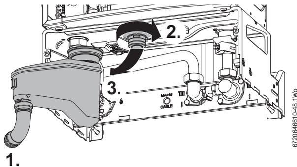
Fig. 71 Siphon removal
