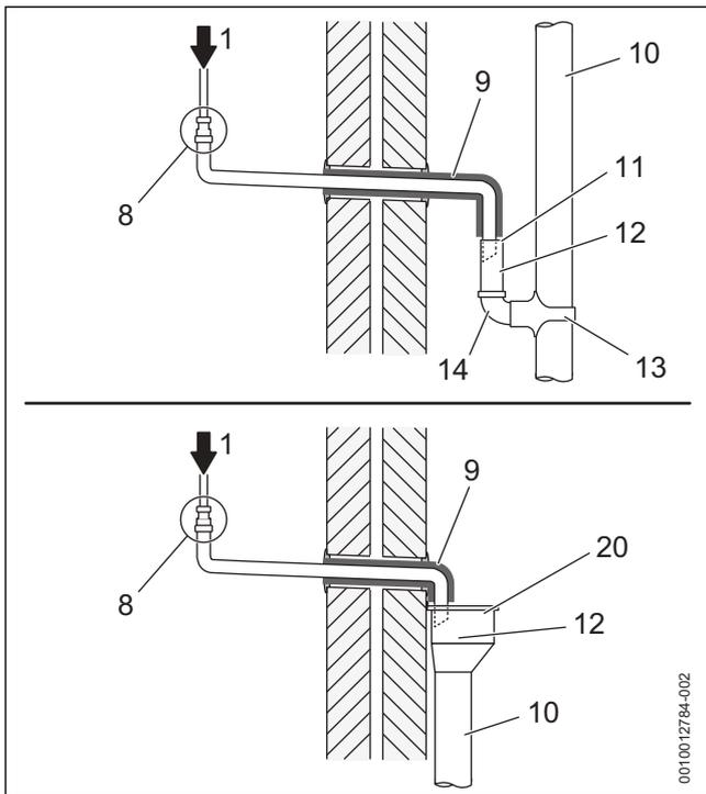
Fig. 32 Disposal into rain water down pipe
