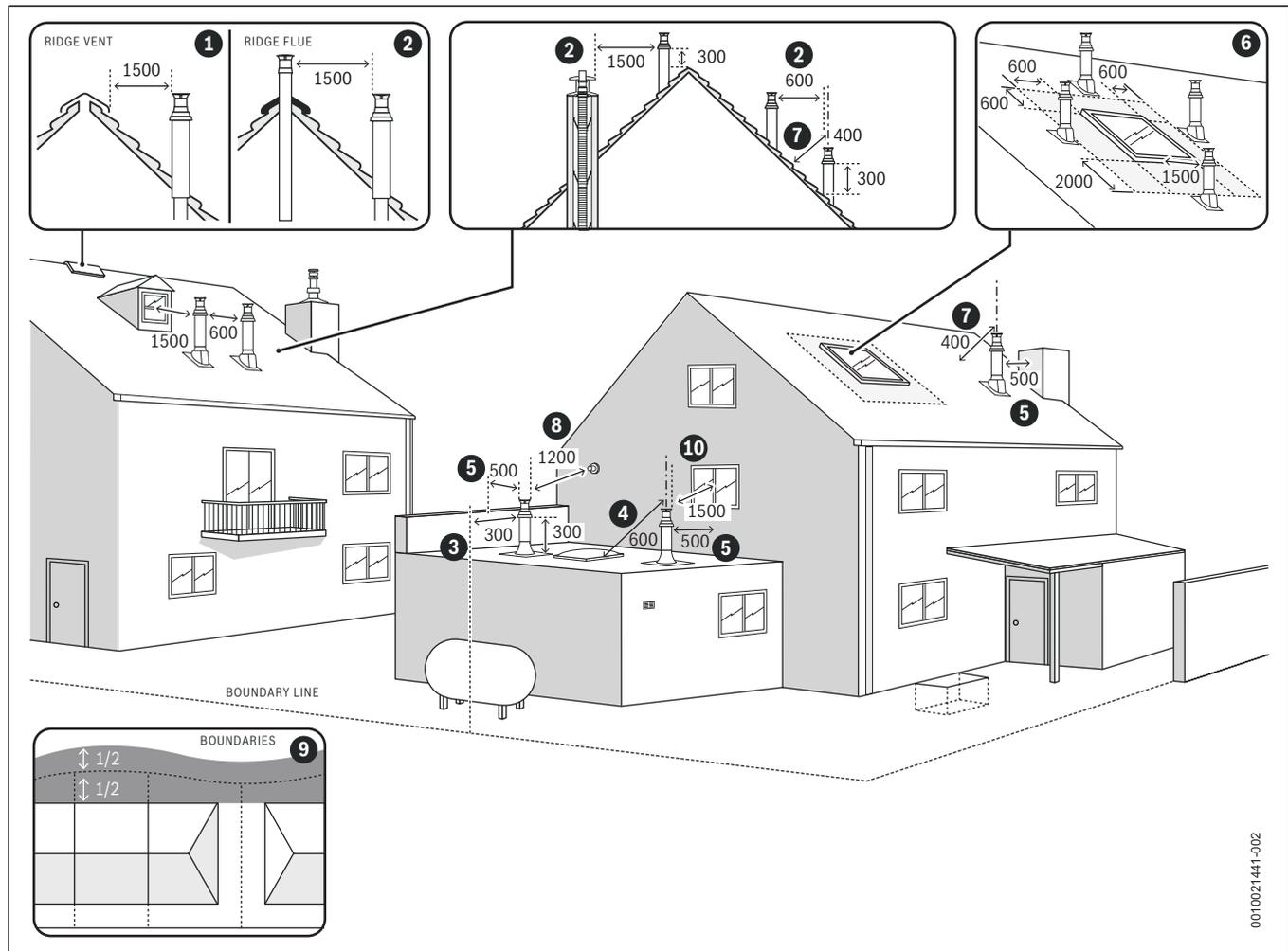
Fig. 26 Vertical flue terminal positions
