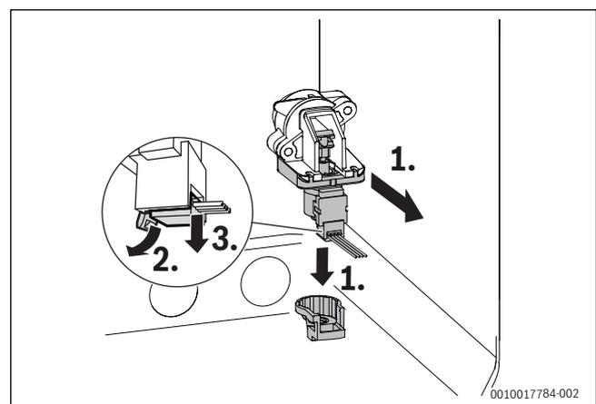
Fig. 102 Removing the motor of the 3-way valve
