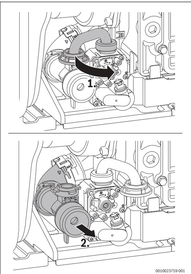
Fig. 78 Venturi removal
