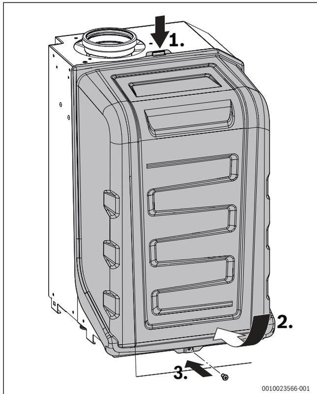
Fig. 63 Refit combustion casing
