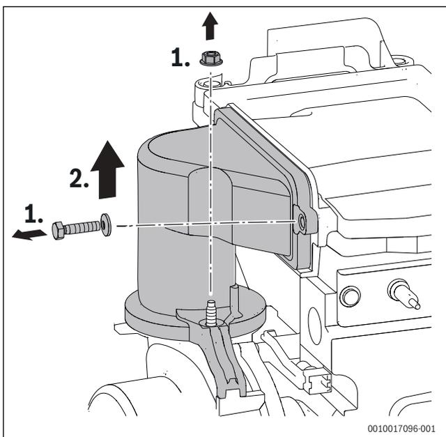
Fig. 76 Removing the air-gas manifold
