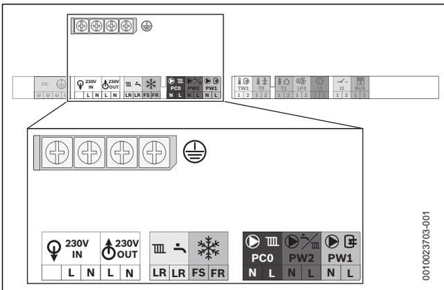
Fig. 52 Power supply (power cables) terminal strip
