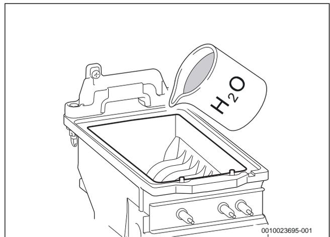
Fig. 83 Pour water into the heat exchanger
