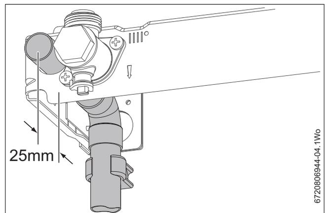
Fig. 43 Fitting the condensate pipes to the mounting plate
