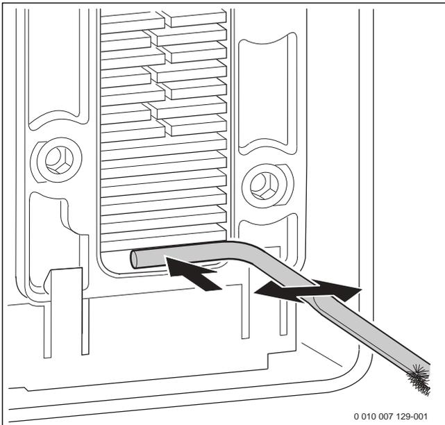
Fig. 84 Cleaning debris
