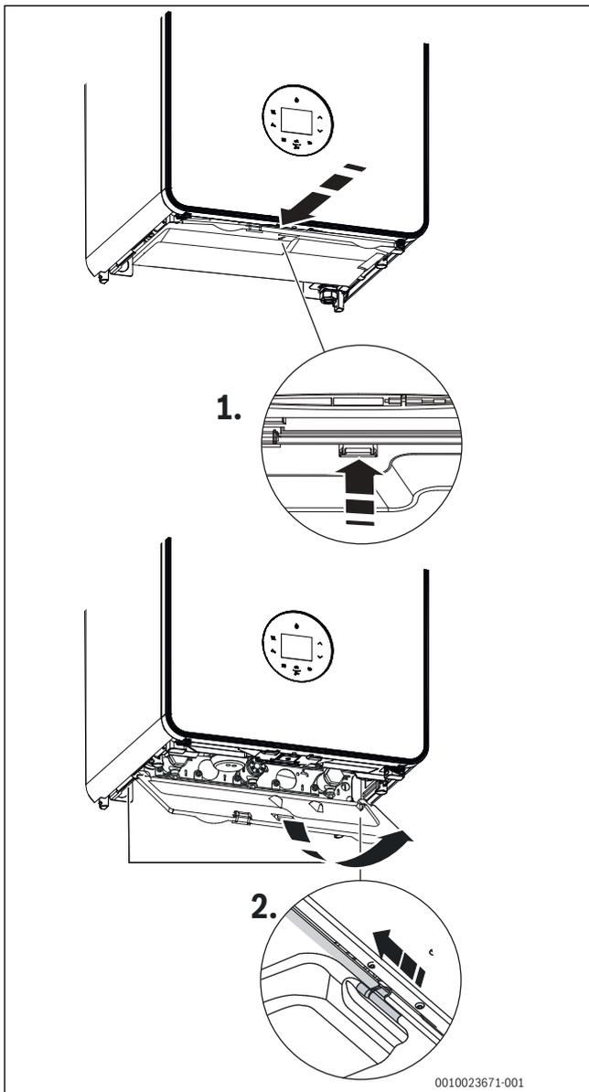
Fig. 70 Removing bottom panel
