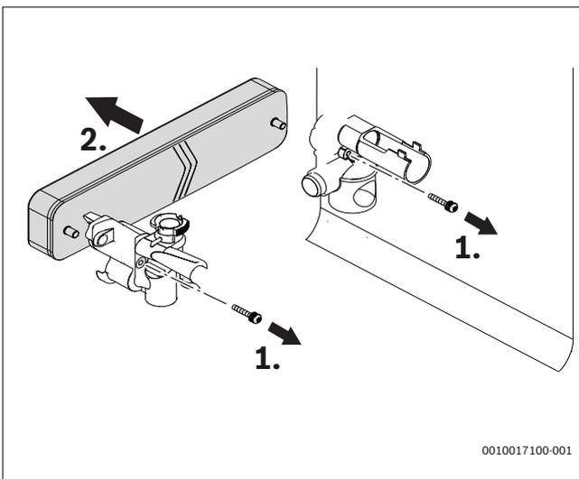
Fig. 104 Removing the plate heat exchanger
