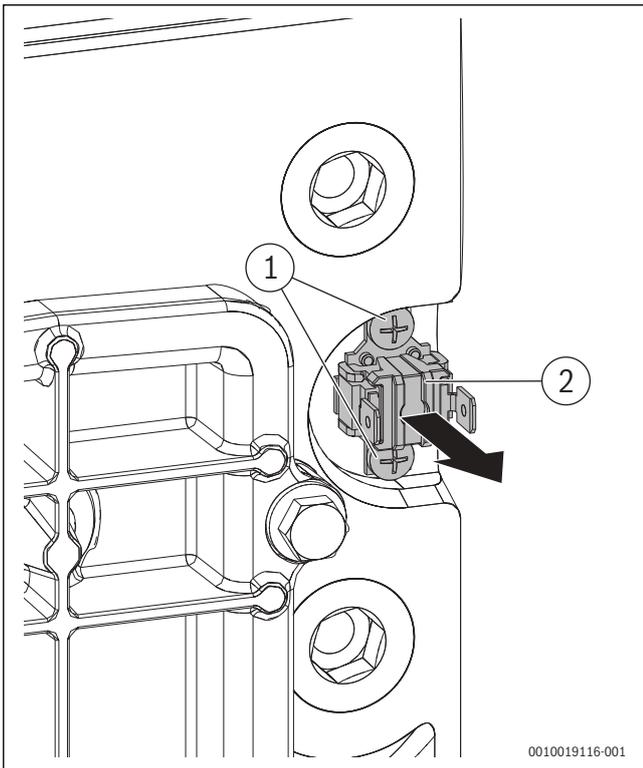
Fig. 96 Removing overheat thermostat
