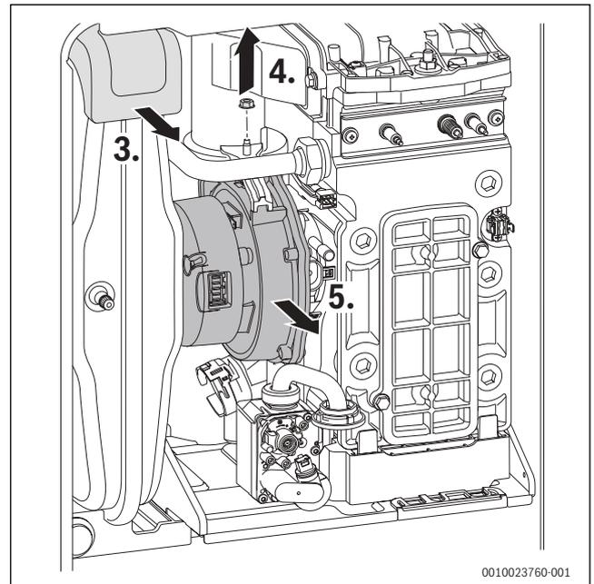
Fig. 79 Fan removal
