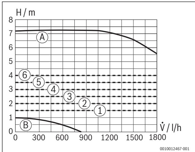
Fig. 105 Pump characteristic maps and pump curves
