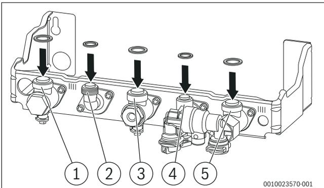
Fig. 41 Fitting the sealing washers
