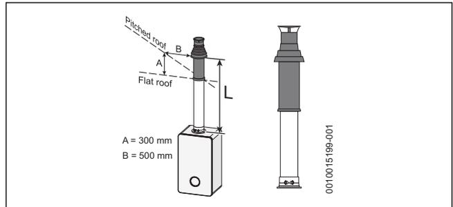
Fig. 21 Vertical flue option
