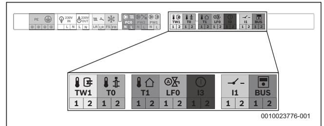
Fig. 53 Low voltage (signal cables) terminal strip
