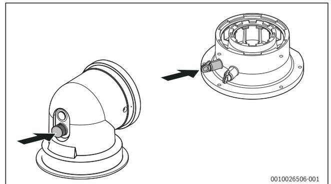
Fig. 94 Flue gas test point
