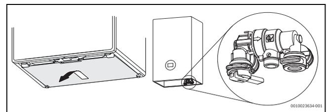
Fig. 3 Enable access to keyless filling link
