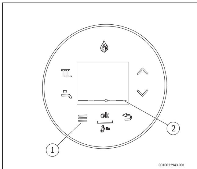
Fig. 2 Pressure indicator for checking the operating pressure
