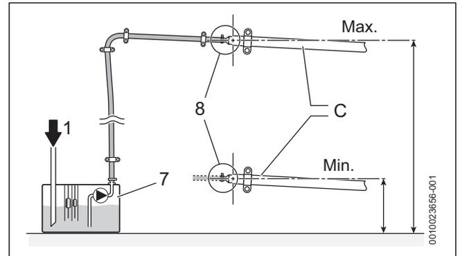
Fig. 31 Condensate pump example
