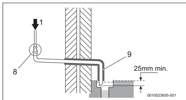
Fig. 33 Disposal to open drain or gully
