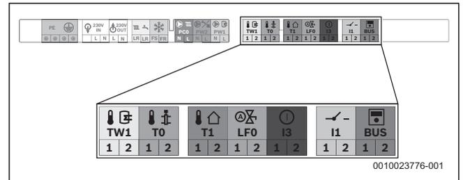
Fig. 54 Low voltage (signal cables) terminal strip
