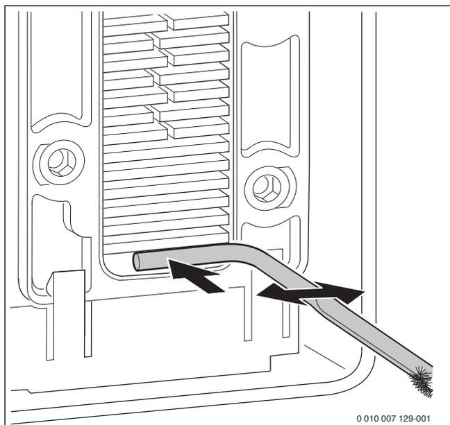
Fig. 86 Cleaning debris
