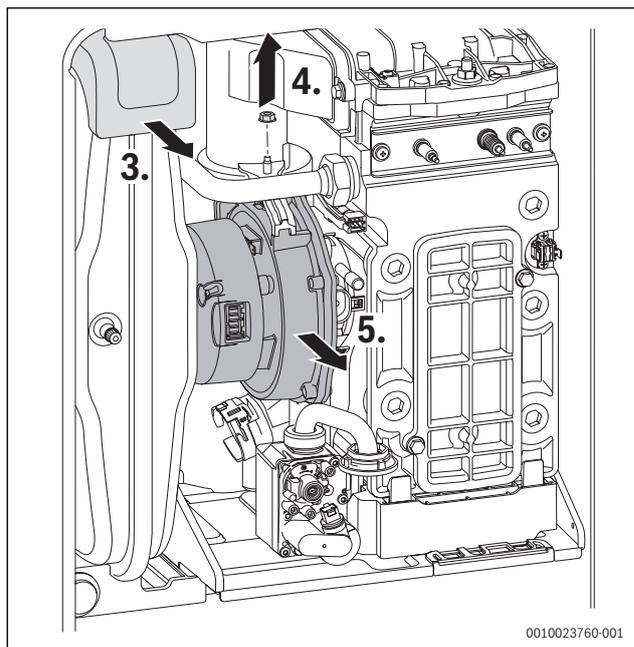
Fig. 81 Fan removal
