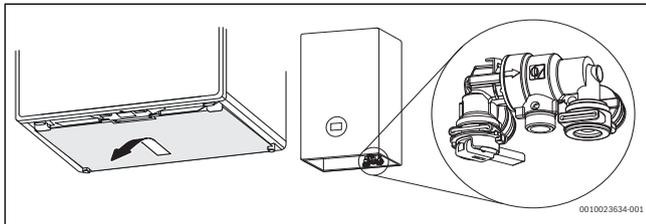
Fig. 59 Enable access to keyless filling link
