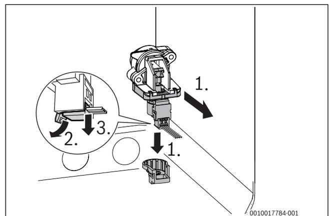
Fig. 104 Removing the motor of the 3-way valve
