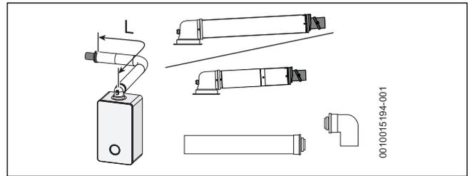
Fig. 16 Horizontal flue option
