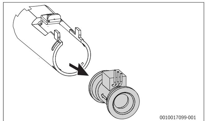
Fig. 103 Removing the flow turbine at the cold water pipe
