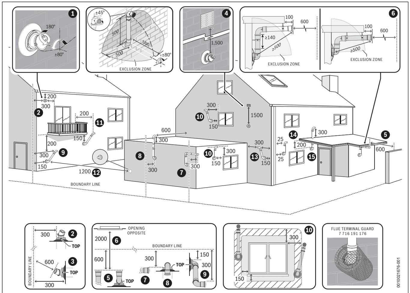
Fig. 28 Plume re-redirect and plume management terminal positions
