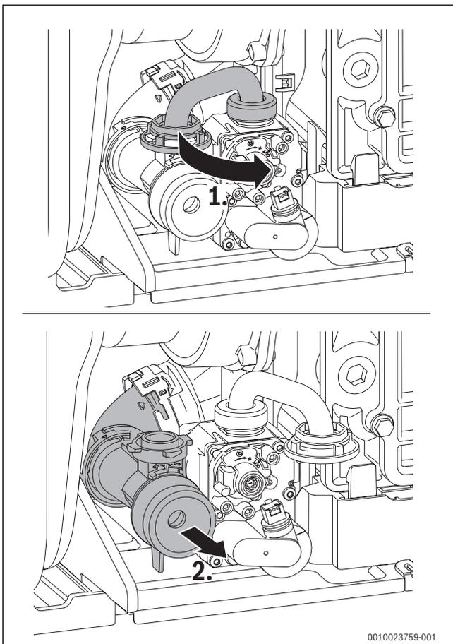
Fig. 80 Venturi removal
