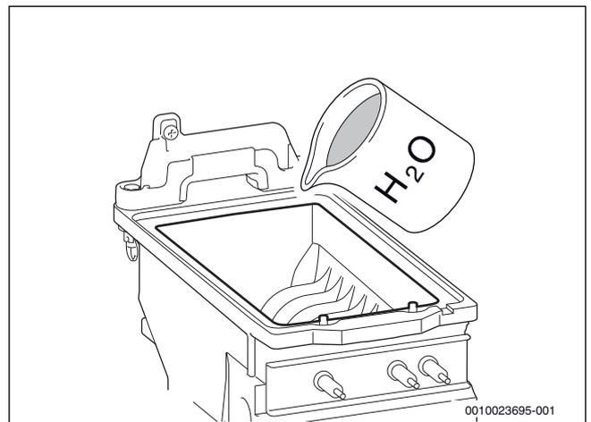
Fig. 85 Pour water into the heat exchanger
