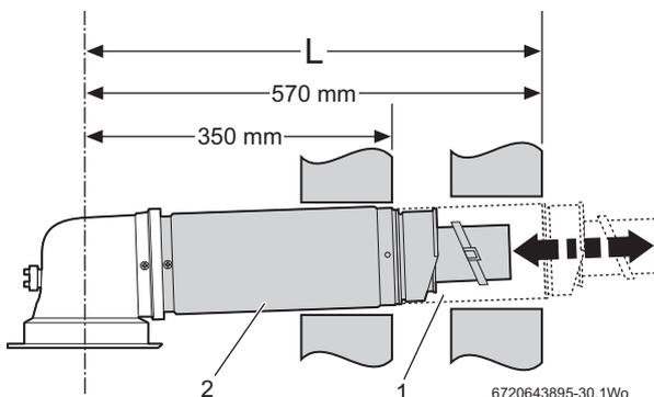
Fig. 31 Standard telescopic flue
