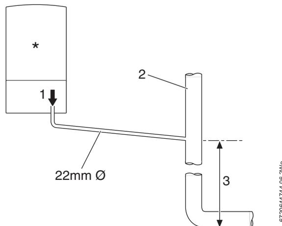
Fig. 8 Disposal to soil vent stack
