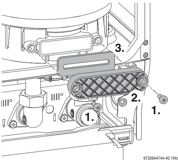
Fig. 67 Access cover removal
