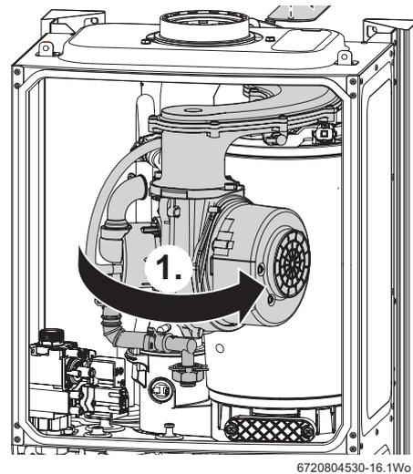
Fig. 79 Rotate the air/gas manifold assembly
