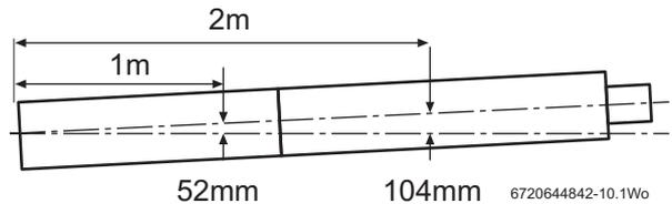
Fig. 36 Slope for condensate disposal
