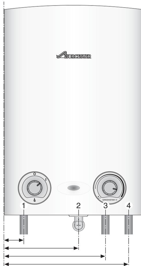
Fig. 19 Pipe work dimensions
