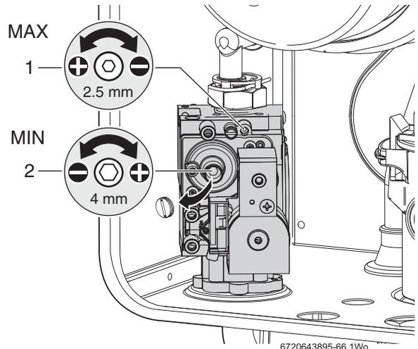
Fig. 61 Gas valve adjustment
