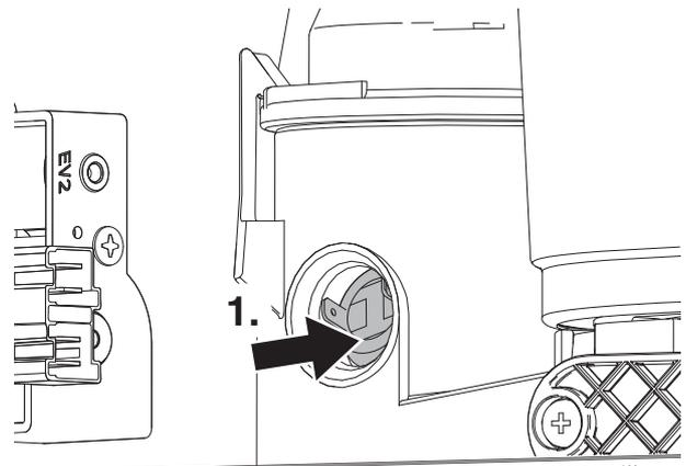
Fig. 74 Remove thermostat
