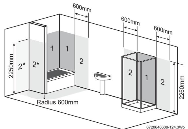
Fig. 17 Bathroom installations
