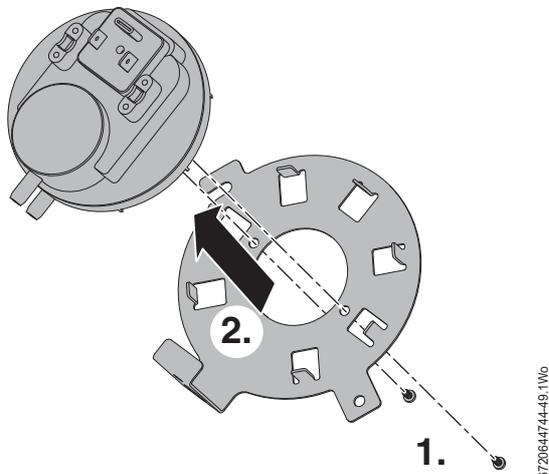
Fig. 81 Air pressure switch bracket
