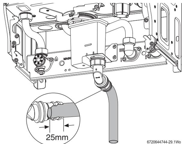
Fig. 43 Condensate connection
