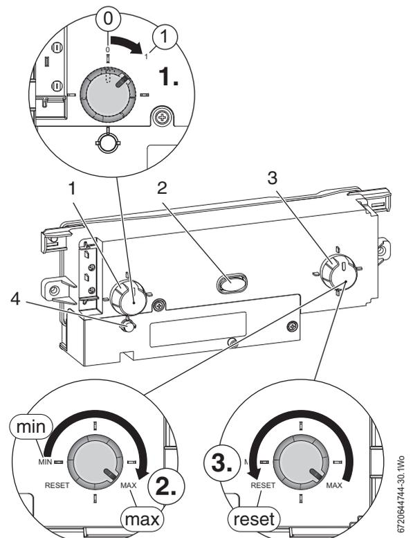
Fig. 45 Boiler controls
