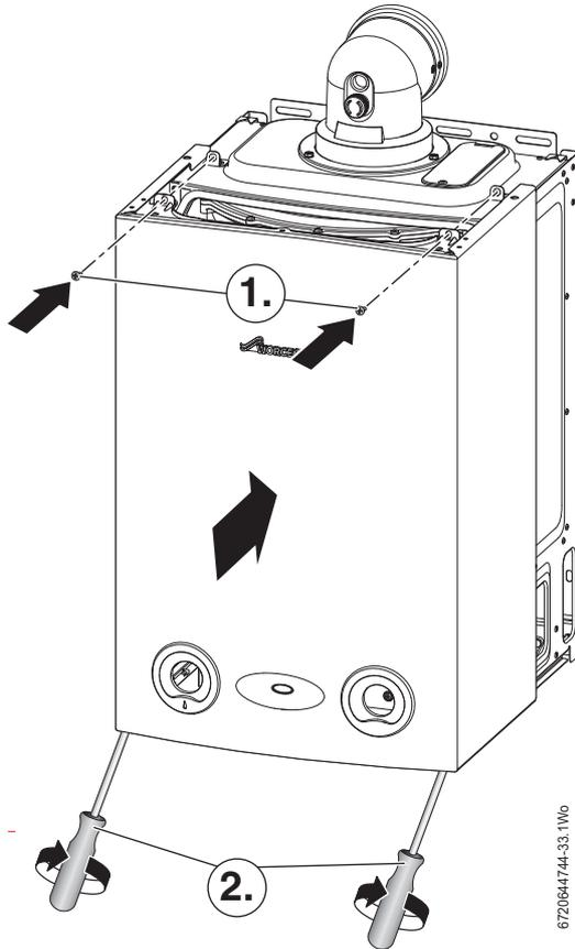
Fig. 50 Replacing outer case
