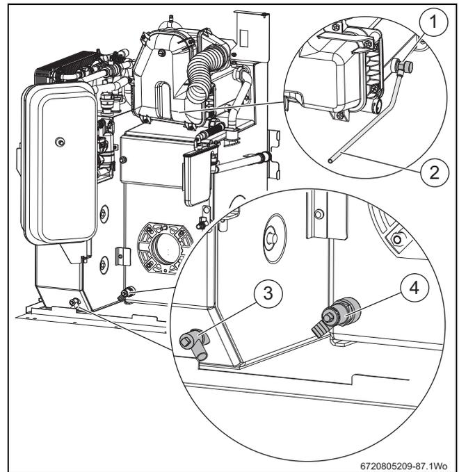
Fig. 67 Appliance drains points
