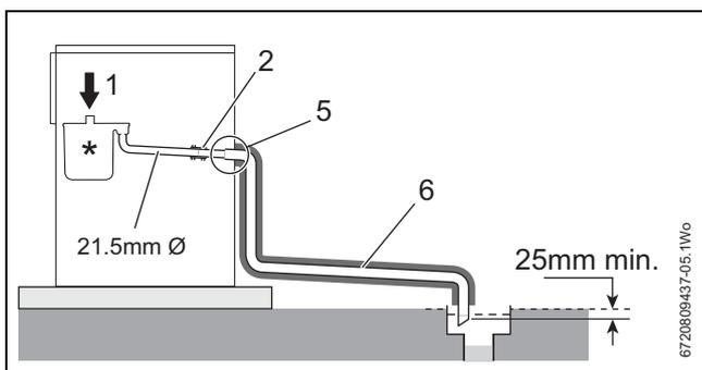
Fig. 13 External drain
