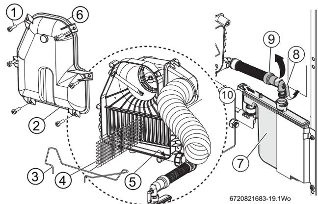
Fig. 75 Secondary heat exchanger and condensate trap detail
