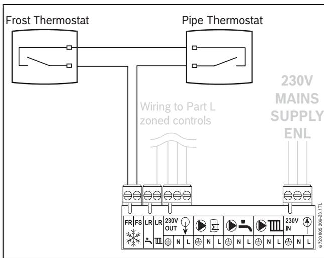
**Fig. 39** Optional External 230 V AC Frost Stat Connection for protection of system pipework in unheated air space
