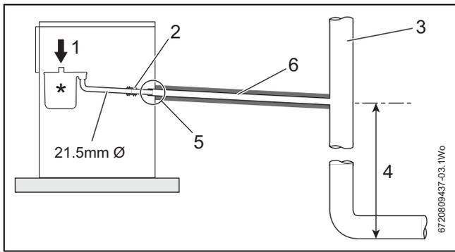
Fig. 11 Disposal to a soil vent stack
