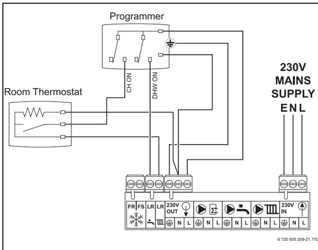
**Fig. 38** External 230 V Twin Channel Programmer and Room Thermostat
