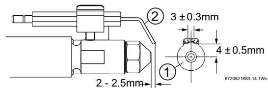
Fig. 33 Nozzle and electrode alignment
