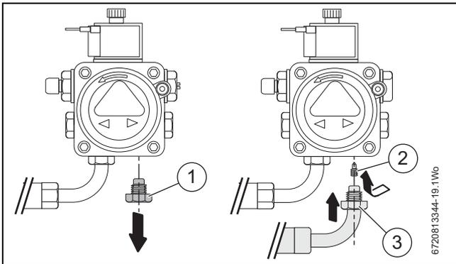
Fig. 34 Converting to double pipe system
