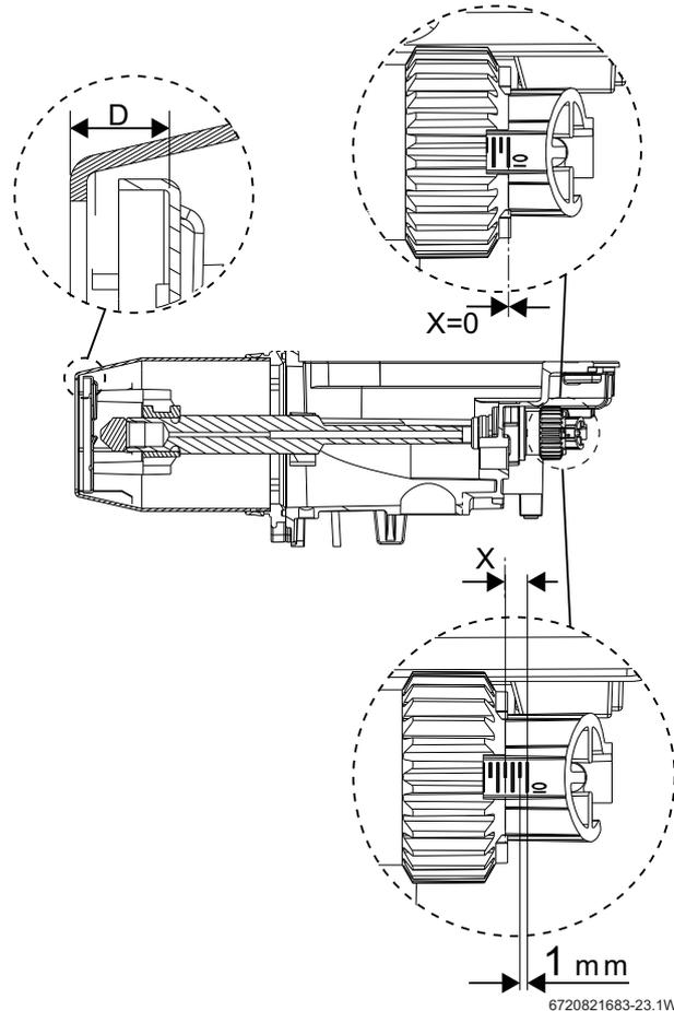
Fig. 53 Burner head adjustment
