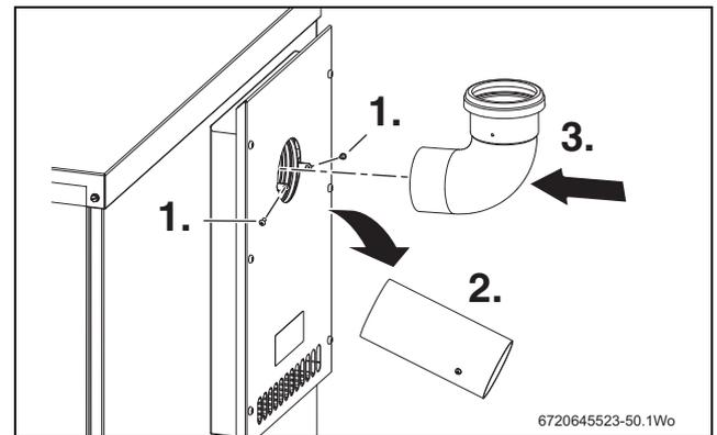
Fig. 22 Fitting the terminal bend
