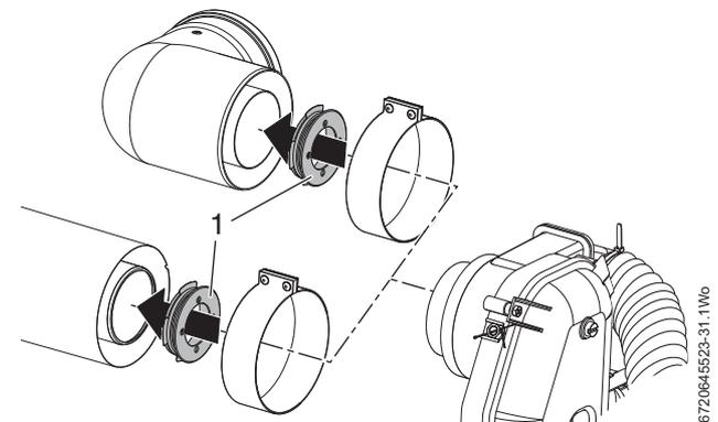
Fig. 27 Flue damper fitting
