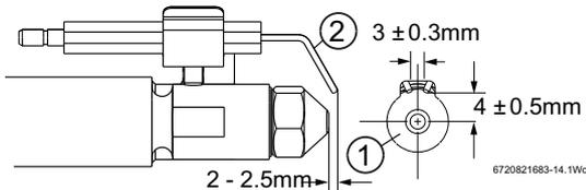
Fig. 73 Nozzle and electrode alignment
