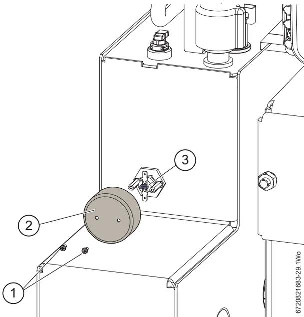
Fig. 95 Tank overheat reset
