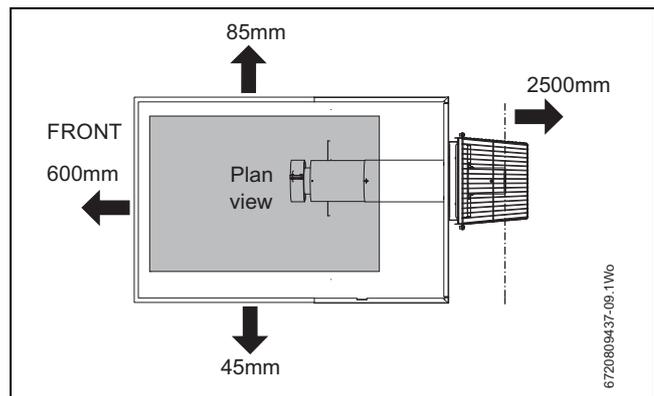
Fig. 17 Rear exit flue clearances
