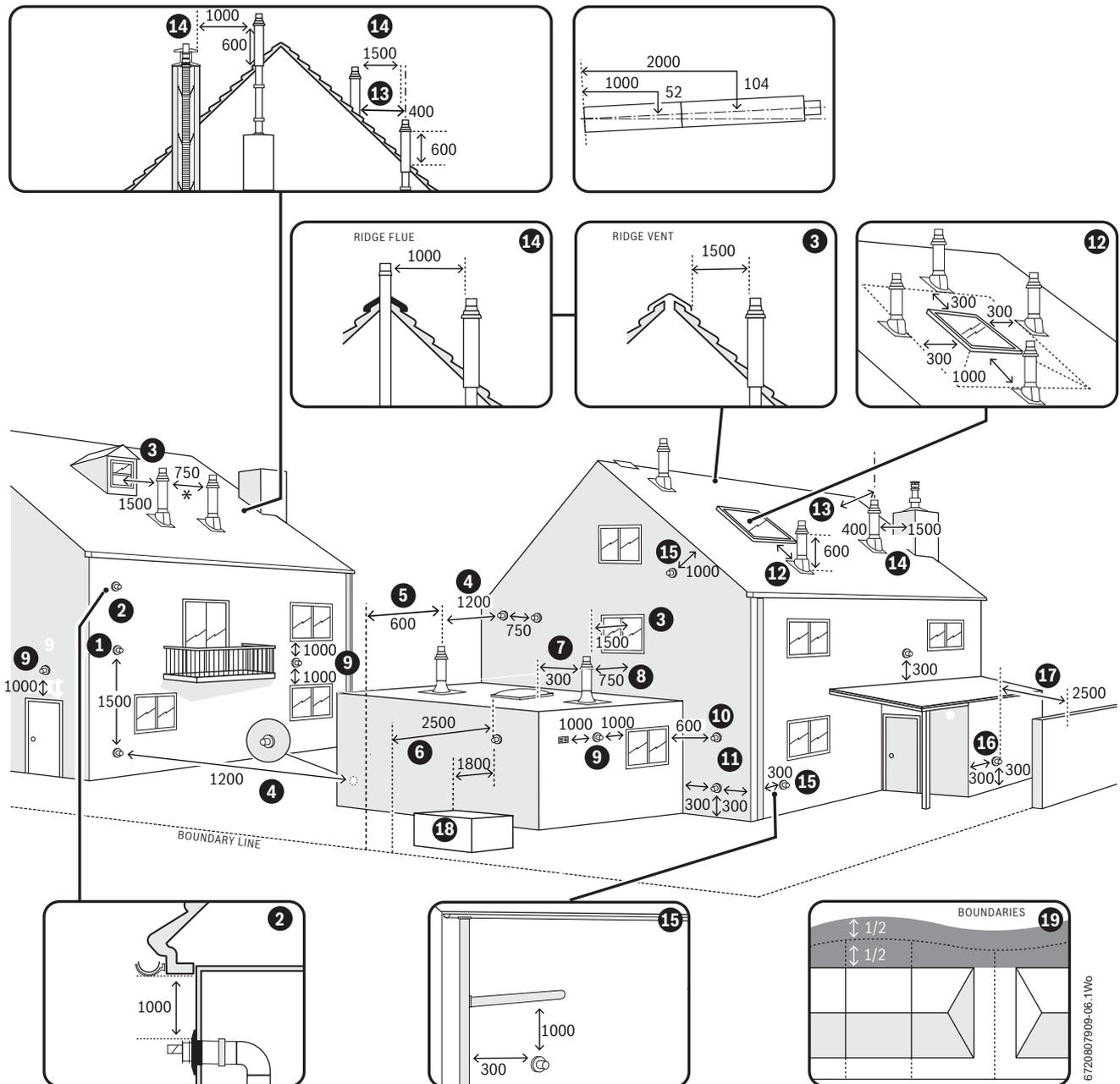
Fig. 20 External boiler flue terminal positions
