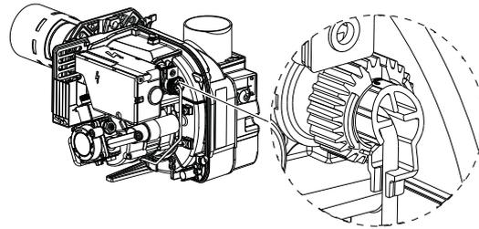
Fig. 52 Burner head adjustment thumbwheel
