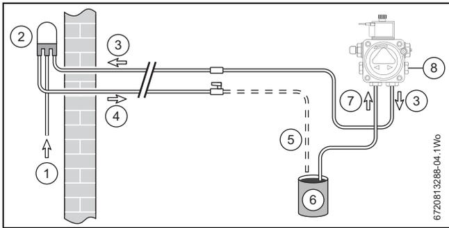
Fig. 50 Priming the pump
