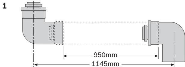
**FLUE MEASURING & CUTTING**
