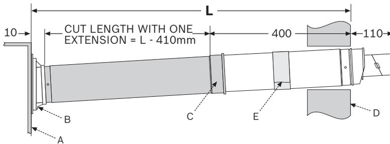
**FLUE MEASURING & CUTTING**
