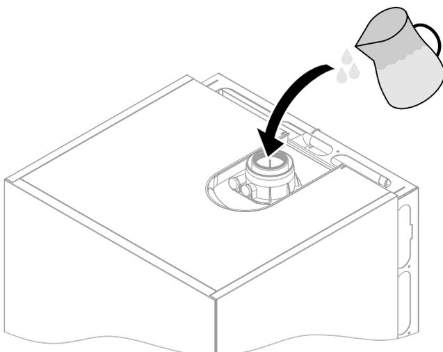
Pour at least 0.3 l of water into the flue gas connection.
