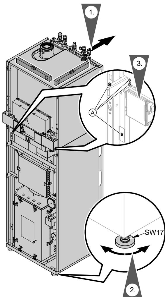
3. Bring the Vitotronic control unit into the maintenance position (see Fig. 53, page 102) and align the side panels using screws (A).
