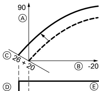
Fig. 47 Example 1: Adjusting the standard set room temperature from 20 to 26 °C
