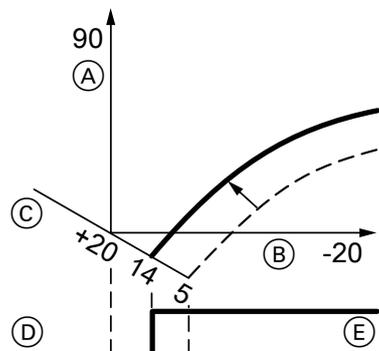
Fig. 48 Example 2: Adjusting the reduced set room temperature from 5 °C to 14 °C
