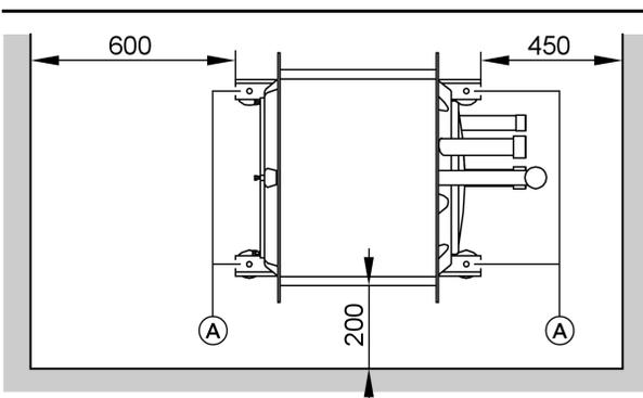
(Boiler body without thermal insulation)
