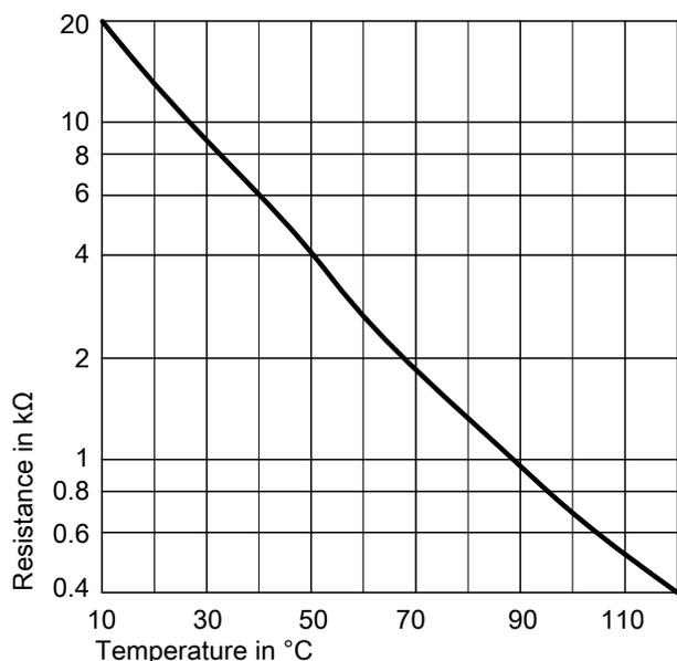
Fig. 51 Sensor type: NTC 10 kΩ
