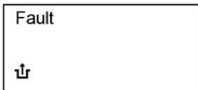
Red fault indicator flashes for all faults.
