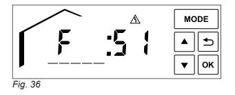
In case of a fault, the display will show  $\underline{\wedge}$  and the fault code.
