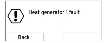
If the controller shows a fault message in the display instead of the basic display and you press the left-hand function key **Back**, then the basic display appears again.
