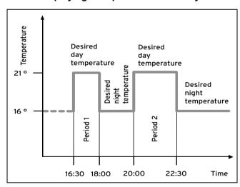
The **Time programmes** function can be used to set the time period for the heating circuit, ventilation unit, hot water generation and circulation pump.
