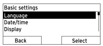
Turn the rotary knob until the **Date/Time** list entry is highlighted.
