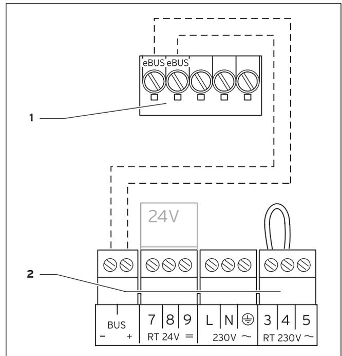
Fig. 5.1 Electrical connection for wireless receiver unit
