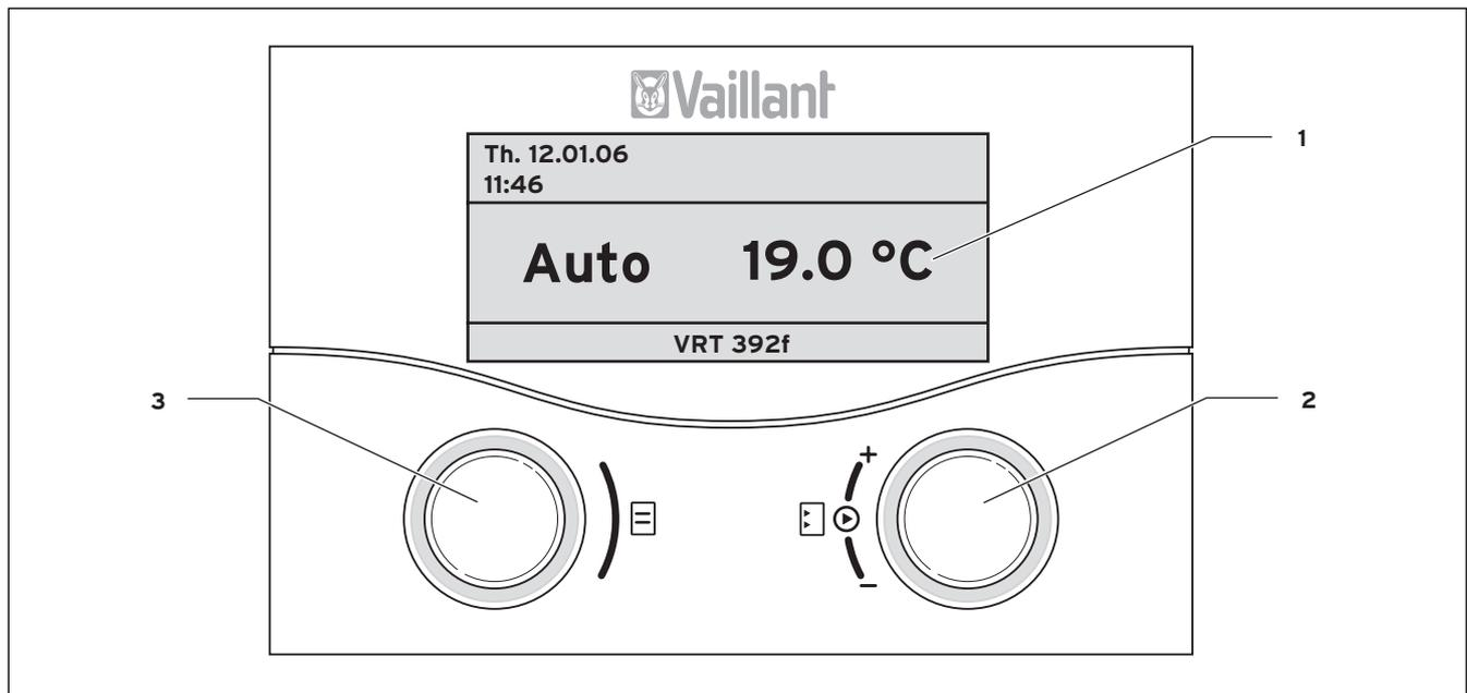
Fig. 4.1 Overview of operator control and display panel
