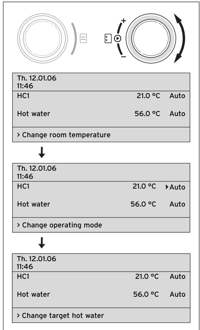
Fig. 4.5 Scroll to various different modifiable parameters
