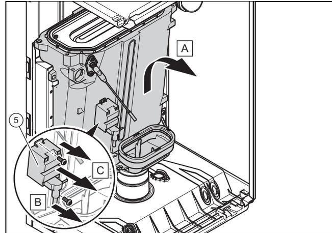
8. Lift the heat exchanger up slightly and remove it together with the condensate tray.
