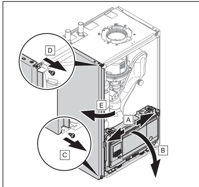
1. Tilt the electronics box forward.
