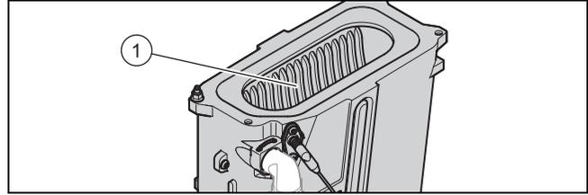
3. Protect the folded down electronics box against sprayed water.
