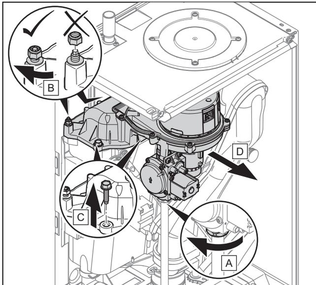
7. Remove the plugs from the gas valve.
