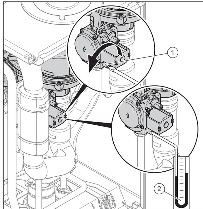
2. Use a screwdriver to undo the sealing screw on the measuring connection (1) of the gas valve.
