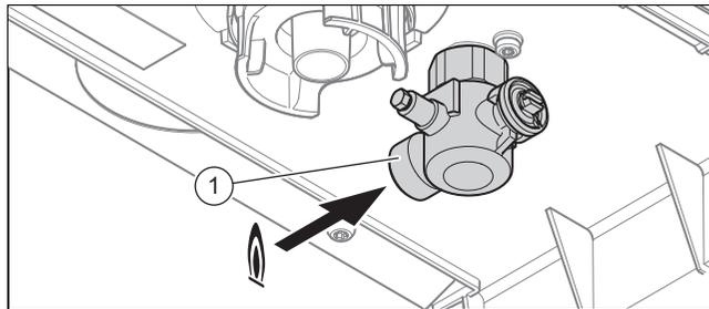
1. Establish the gas connection (1) in accordance with the applicable standards.
