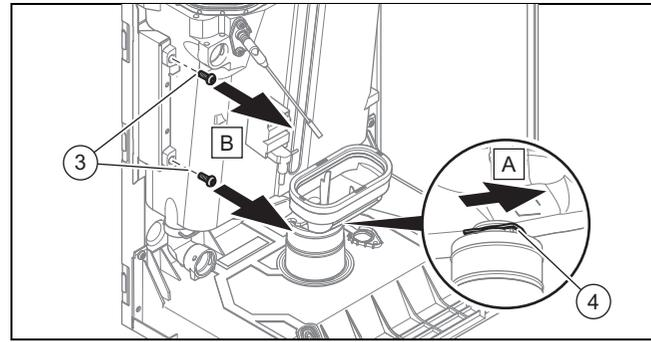
6. Undo the clip underneath the condensate tray (4).
