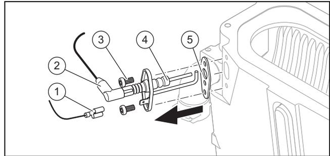
1. Disconnect the connection (2) and the earthing cable (1).
