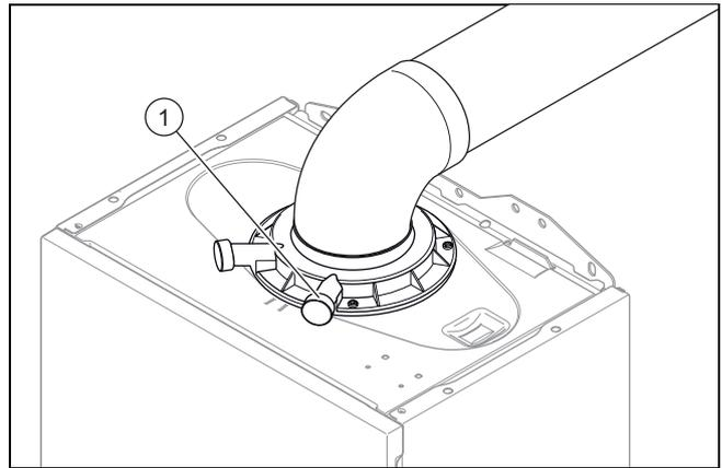
3. Unscrew the cover from the flue gas analysis point (1).
