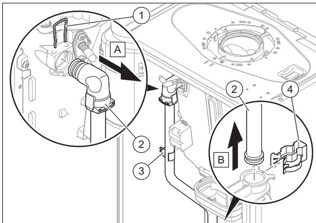
4. Remove the temperature sensor (3).
