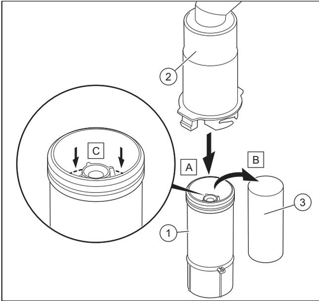
1. Unclip the lower section of the condensate trap (1) from the upper section of the condensate trap (2).
