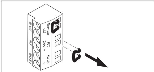
► Remove the bridge from the **24V=RT** plug.
