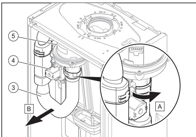
7. Remove the air intake pipe (3).
