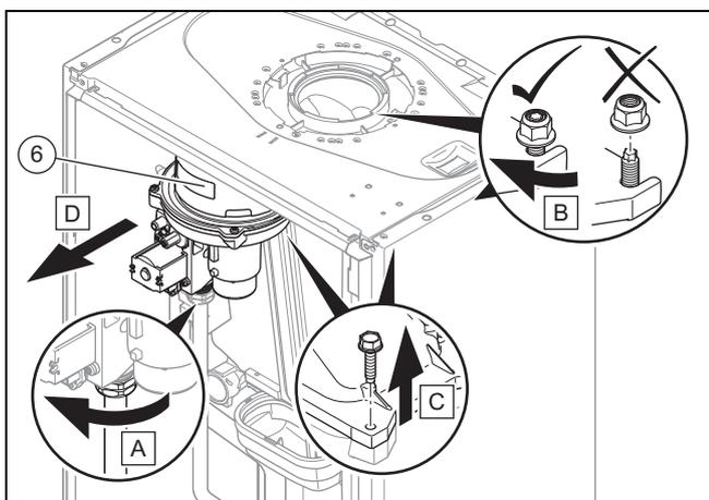
9. Remove the gas-air mixture unit (6).
