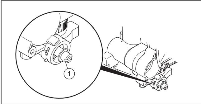
2. Regulate the pressure using the adjusting screw (1).
