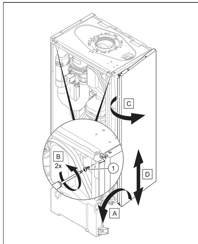
1. Tilt the electronics box forward.
