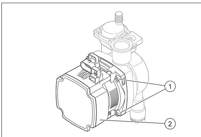
1. Disconnect the pump cable from the electronics box.
