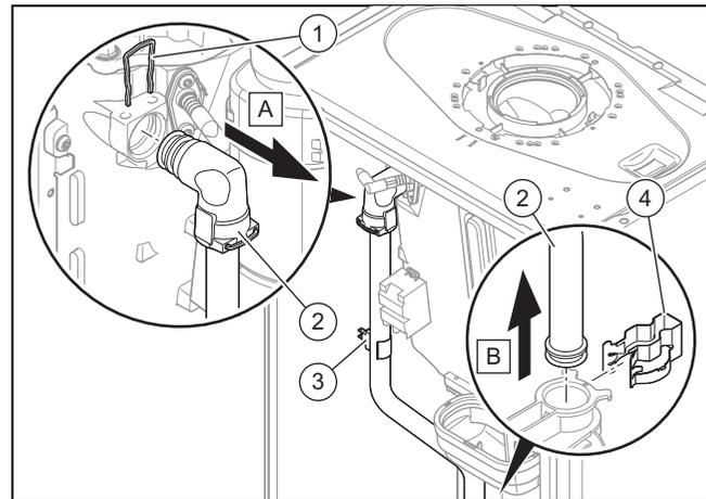
4. Remove the temperature sensor (3).
