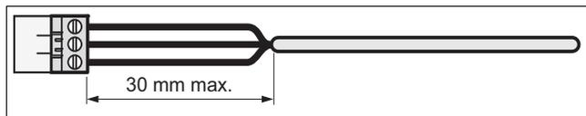
1. Shorten the connection cables to the appropriate lengths to prevent them from causing damage inside the electronics box.
