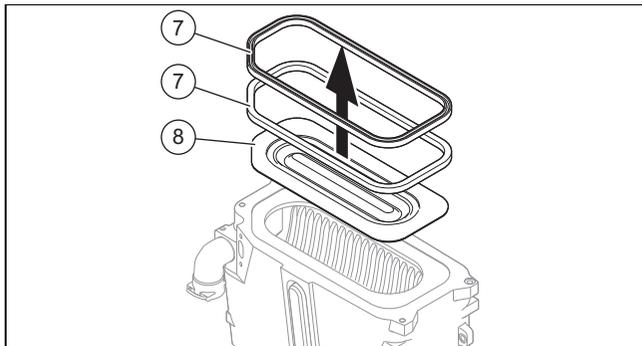
10. Remove the burner seals (7) and the burner (8).
