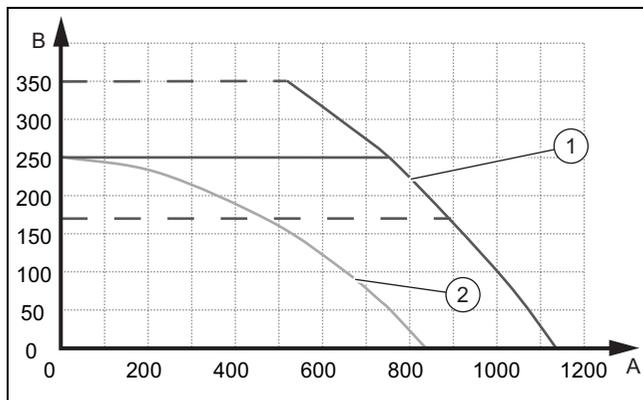
A Remaining feed head [mbar] 1 Max. PWM
