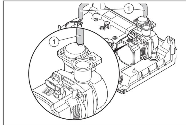
1. Check the silicone hose connection (1) between the pump's automatic air vent and the hydraulic console.
