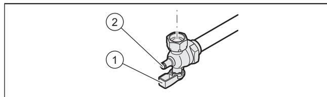
1. Ensure that the gas inlet working pressure can be obtained with all other gas appliances in the property working.
