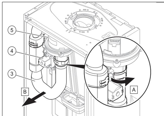
7. Remove the air intake pipe (3).
