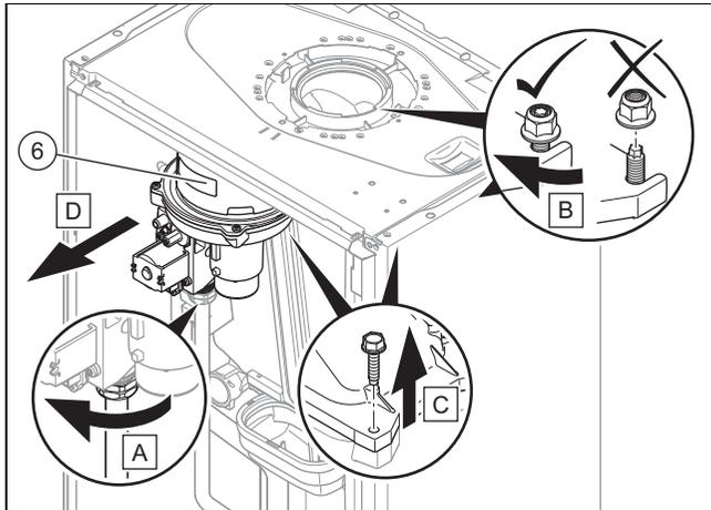
9. Remove the gas-air mixture unit (6).
