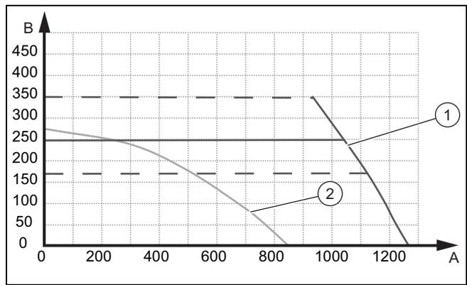
A Remaining feed head [mbar] 1 Max. PWM
