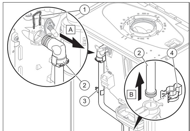
4. Remove the temperature sensor (3).
