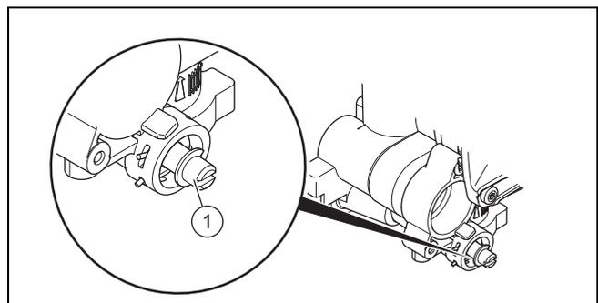
2. Regulate the pressure using the adjusting screw (1).
