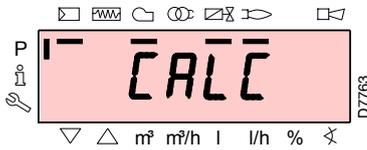
After adjusting point “P1”, press the key “+”: the display shows “CALC” for a few seconds. The control box will automatically calculate the points from “P2” to “P8”, distributing them in a straight line, assuming for point “P9” the factory setting (see the table below). These are theoretical and must be checked.
