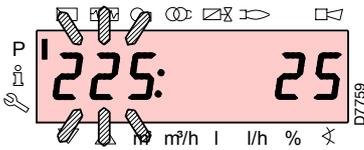
To return to the list of parameters, press simultaneously the keys “+” and “-” (esc).
