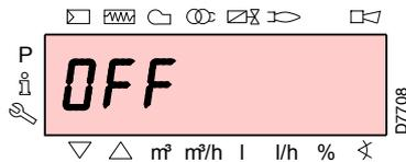
The burner is in the request for heat waiting mode, or the selector "0-1" of Fig. 28 is at the "0" position.
