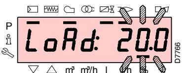
Press the key “F” for 1 second: “LoAd” is displayed and the load percentage flashes.
