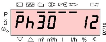
The display visualises the various phases of the start-up, ignition and switch-off of the burner. In the example alongside, the display indicates that the burner is in phase 30 (see the diagram of Fig. 34) and there are 12 s until the next phase.
