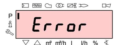
If the password inserted is incorrect, the message "Error" will appear for a moment.
