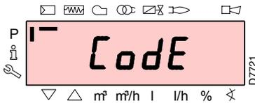
Press the keys "F" and "A" simultaneously for 1s: for a moment the display will show "CodE", and immediately after you will see 7 dashes, the first one flashing.
