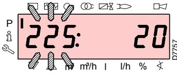
After accessing the level and group of parameters, the display visualises the number of the parameter (flashing) on the left, and the corresponding value on the right.
