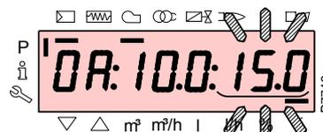
For the air servomotor, keep the key “A” pressed (the position in degrees flashes) and press the keys “+” or “-” to increase or decrease the value.
