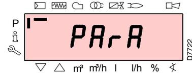
Select the group of parameters with keys "+" and "-", and confirm by pressing the "i/reset" key.
