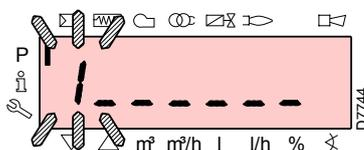
With the keys "+" and "-" select the first character of the password (letter or number), and confirm by pressing the key "i/reset".
