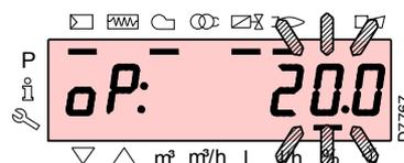
Releasing the key “F”, the standard visualisation appears, with the current load percentage flashing: this means that the burner is working in manual mode (any outside adjustment is excluded and only the safety devices are active).
