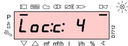
The burner is in lockout when the red indicator light on the Operator Panel is switched on and the display visualises alternately the lockout code (in the example alongside **c: 4**) and the relative diagnostic (in the example **d: 3**).
