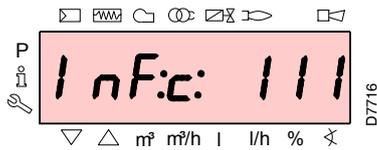
The display visualises alternately an error code and a diagnostic, which does not take the system into safety mode.
