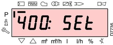
Access the Parameters Level referring to “Access procedure with password”. The display visualises the parameters group **400**; confirm with the key “i/reset”.
