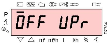
Check that the display of the Operator Panel shows request for heat and “OFF UPr”: this means it is necessary to set the modulation curve of the burner.
