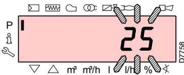
Press the key “+” and increase the value to 25 seconds (flashing). Press the key “i/reset” to confirm and store.
