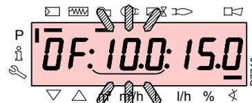
For the fuel servomotor, keep the key “F” pressed (the position in degrees flashes) and press the keys “+” or “-” to increase or decrease the value.
