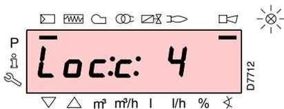
The burner goes into lockout.
