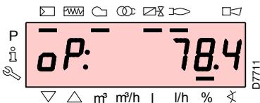
The burner is working in the requested load position (in the example alongside, **78.4%**).
