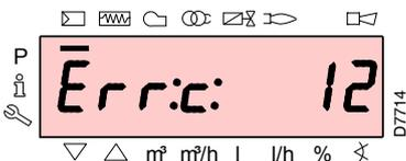
The display visualises alternately the error code (in the example alongside, **c: 12**) and the relative diagnostic (in the example **d: 0**).
