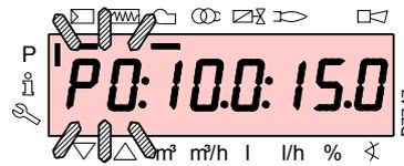
Using the keys “+” and “-” insert/select the curve point you want and wait for it to flash: this means that the servomotors are now positioned on the values shown on the display and which correspond to the point previously set.
