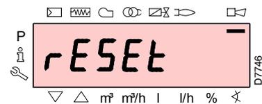
To reset, press the “i/reset” key for 1s: the display will show “rESEt”. When the key is released, the lockout signal will disappear and the red indicator light will switch off. The control box is reset.
