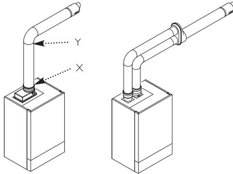
**NOTE:** Horizontal flue pipes should always be installed with a 1.5° fall from the terminal to allow condensate to run back to the boiler.
