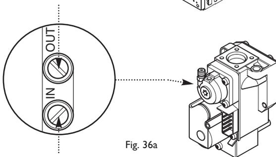
Inlet Gas Pressure Test Point
