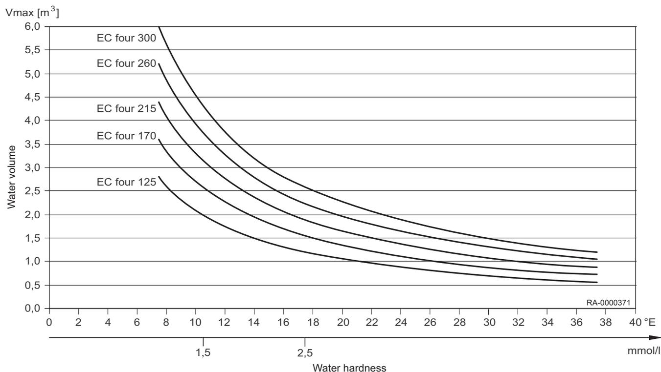
**Description:** The boiler type, the water hardness and the water volume of the heating system must be known. If the volume is above the curve, a partial softening of the tap water or addition of hardness stabiliser is required.
