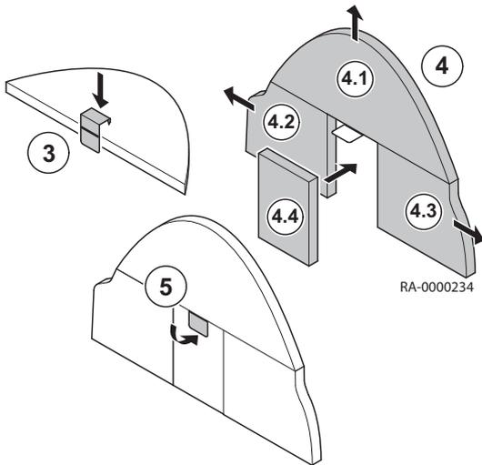
3. Insert a retaining clip with the angled tips from behind into the upper insulating panel
