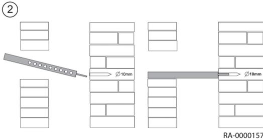
Fig.26 Insertion into the duct
