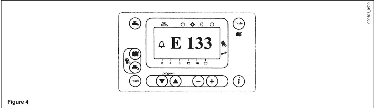
Fault warnings appear on the secondary display (figure 1 b) alternating with the time, both of them flashing (figure 4.1). It is not possible to reset malfunction warnings which appear on the secondary display as the cause of the alarm has first to be removed.
