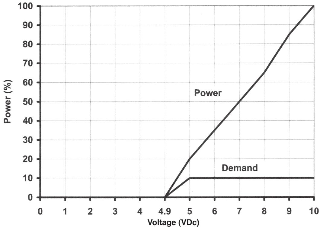
Boiler heating performance according to the voltage on the connector (with voltage above 5V).
