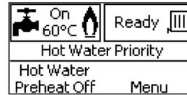
2. Fully open a DHW tap and check that hot water is delivered.
