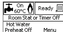
6. Check the correct operation of the timer (if fitted) and all other system controls. Operate each control separately and *Note. The temperature displayed "XX°C" is that measured at that moment, not the set temperature.*
