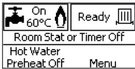
2. Close all taps except the furthest one from the boiler and check that the boiler is firing at maximum rate. This is factory set to give a DHW temperature rise of approximately 35°C at the flow rate stated on page 10 under "operation".
