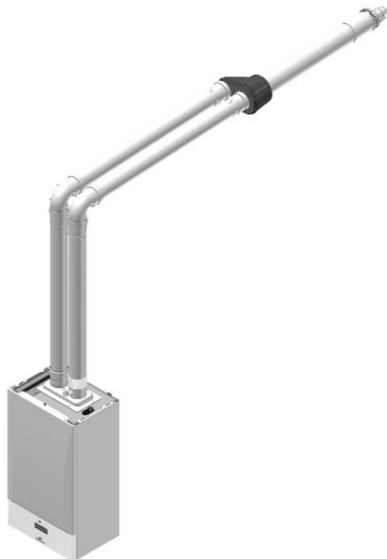
Fig.3-14 Offset Twin to Horizontal Concentric Terminal
