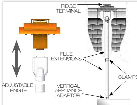
FIGURE 10. OPTIONAL ROOF OUTLETS
