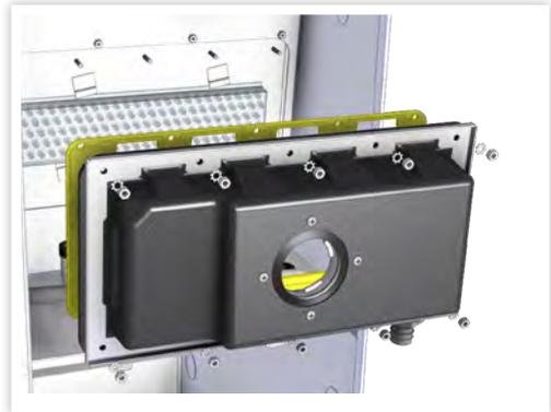
FIGURE 21. COMBUSTION AIR PASSAGE REMOVAL
