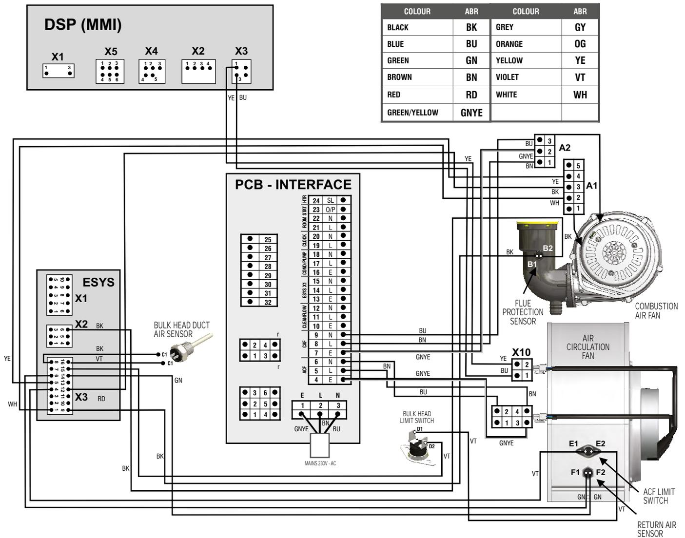
FIGURE 33. WIRING DIAGRAM No. 2 WIRING ROUTING TABLE
