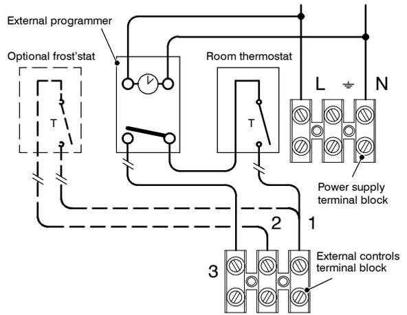
**N.B. These diagrams are schematic only and do not show external terminal strips etc.**
