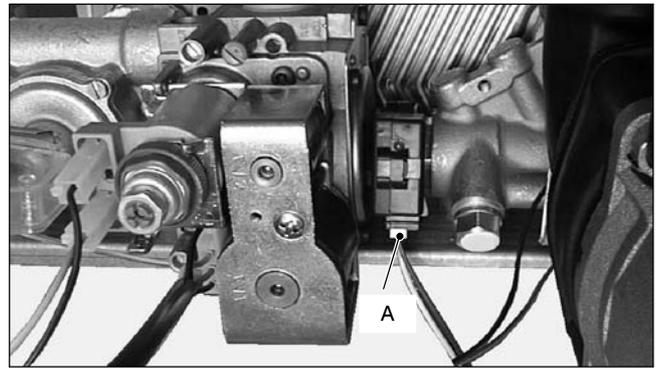
**58 DHW FILTER AND FLOW LIMITER REPLACEMENT**
