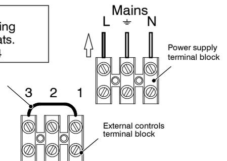
*Note: Ensure that the lengths of the current conductors are shorter than the earth conductor so that if the cable slips in its anchorage the current carrying conductors become taut before the earth conductor.*
