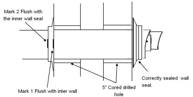
*Note. If the 2 location marks are not visible then the flue is not pulled back far enough to obtain the correct seal. If the 1st location mark has passed the face of the wall the flue has been pulled too far back and the outer wall seal will have been dislodged from its mounting and will need to be refitted.*
