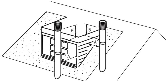
If chimney penetrates dotted area such that A is less than 300mm, B shall not be less than 300mm.
