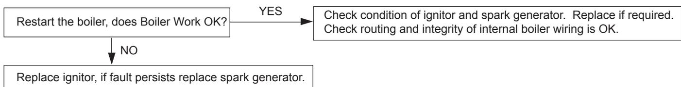
**RESTART PROCEDURE:** To restart boiler press the restart button.
