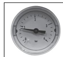
**THE BOILER WILL NOT OPERATE IF THE PRESSURE HAS REDUCED TO LESS THAN 0.3 BAR UNDER THIS CONDITION.**
