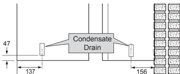
This appliance is fitted with a siphonic 75mm condensate trap system that requires filling before operating the appliance for the 1st time or after maintenance.
