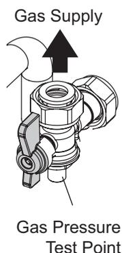
**As part of the commissioning process, the combustion of this appliance must be checked and the Benchmark Checklist completed. A flow chart to assist is provided on page 69.**
