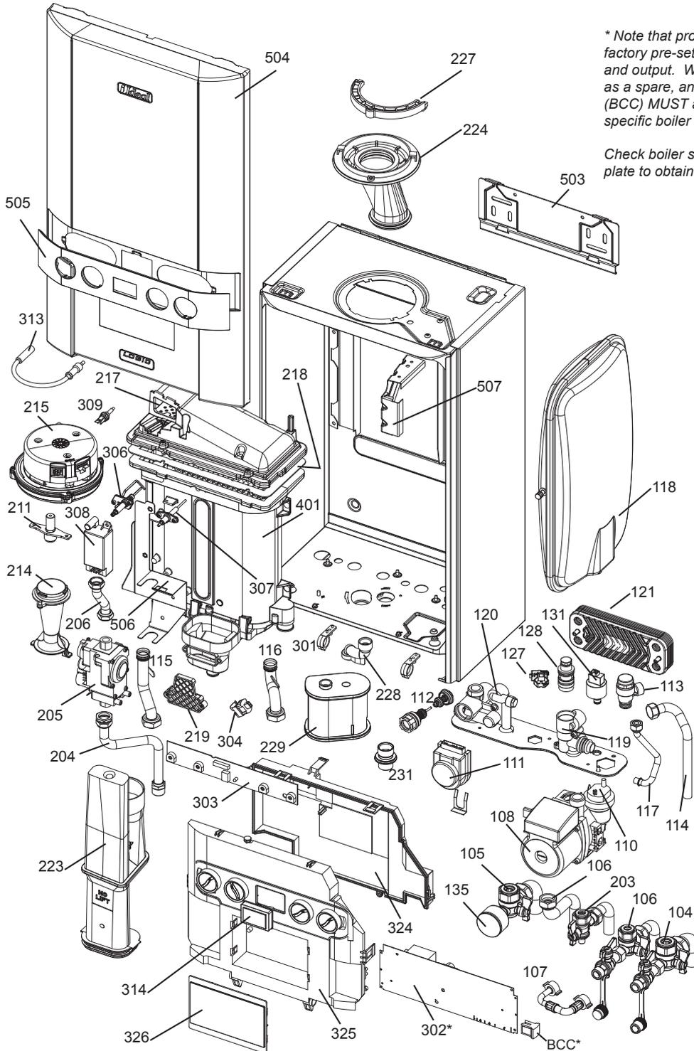
\* Note that production boiler PCBs are factory pre-set to operate for boiler range and output. When ordering Primary PCB as a spare, an additional Boiler Chip Card (BCC) MUST also be purchased for your specific boiler range and output.
