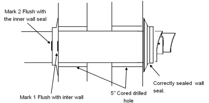
*Note. If the 2 location marks are not visible then the flue is not pulled back far enough to obtain the correct seal. If the 1st location mark has passed the face of the wall the flue has been pulled to far back and the outer wall seal will have been dislodged from its mounting and will need to be refitted.*
