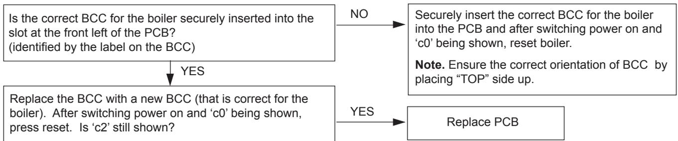
**RESET PROCEDURE** - To reset boiler, turn mode knob to reset position and immediately turn knob back to required setting.
