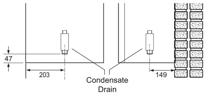
This appliance is fitted with a siphonic 75mm condensate trap system that requires filling before operating the appliance for the 1st time or after maintenance.
