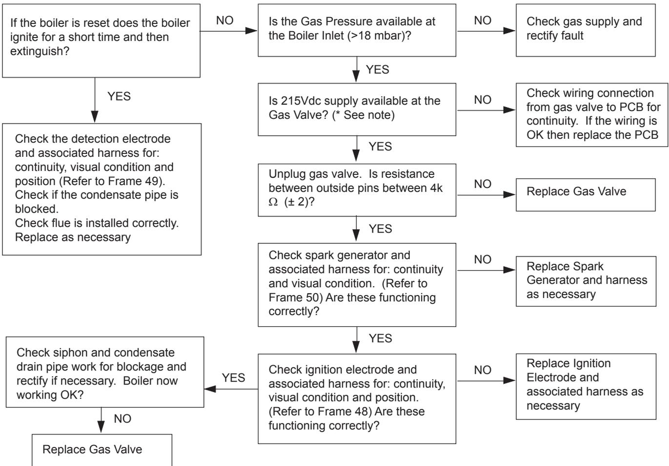
\* **Note:** due to the wave form of the rectified voltage, the reading will vary depending on the type of meter used to measure the value. In general terms a reading greater than 150V indicates that the correct voltage is supplied to the gas valve.
