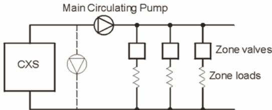
When the clock period ends, Zone valve 1 will (stay) open via normally closed relay contacts to achieve pump overrun.
