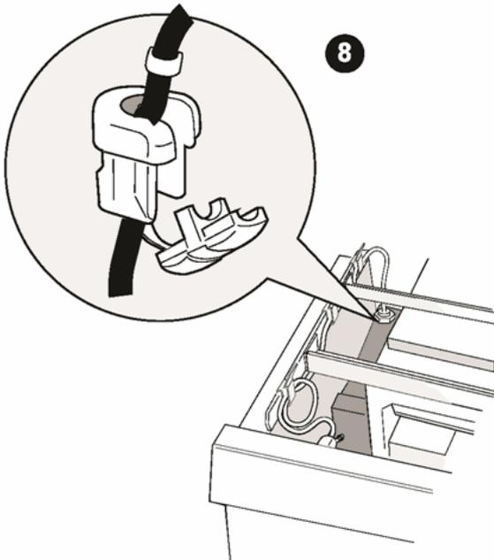
Fit the plastic Heyco bush over the sensor lead at the line shown and insert it into the thermostat pocket. Ensure that the Heyco bush is correctly located.
