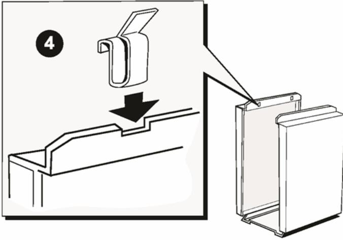
5. Fit the spire clips to the side casing panels.
