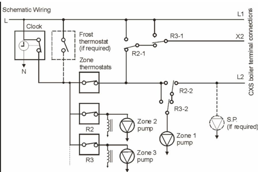
NB. Contacts shown at room temperature with power off
