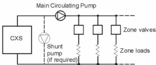
At the start of the next call for heat (or the next clock period) valves on zones not calling for heat will motor shut.
