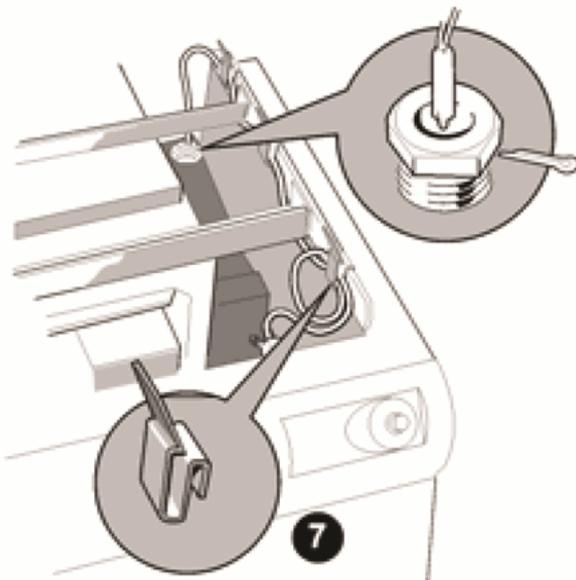
Ensure the phial is correctly seated in the correct pocket opposite side to the flow connection. Refer to [Frame 9](#). Secure with the split pin provided.
