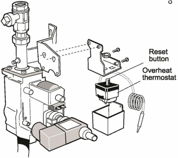
**34 CONTROL BOX - Basic Boiler, Exploded View**
