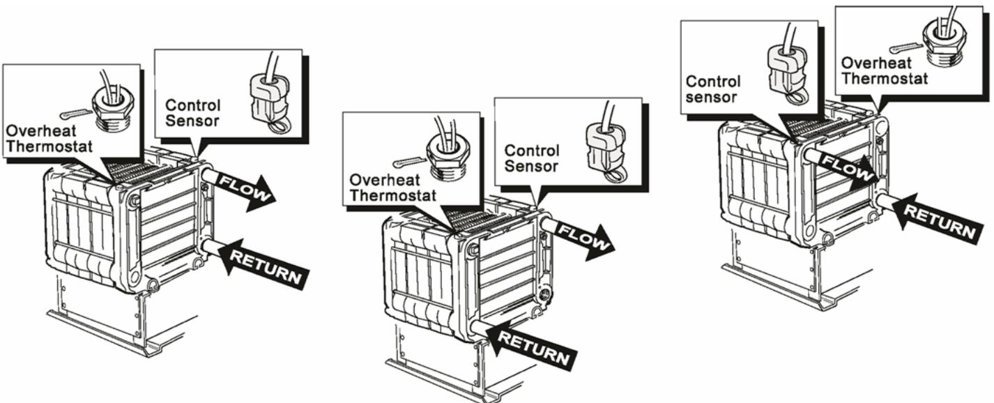
Position the overheat thermostat phial into the thermostat pocket at the opposite side to the flow pipe. The illustrations below show the rear of the boiler with the flow and relative overheat thermostat positions.
