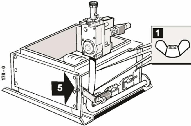
18. Insert the burner rear supports into the slots at the back of the combustion chamber. Lift the front of the burners over the injectors and pull forward to engage.
