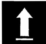
This Way Up: The box must be stored in the position that this arrow shows up.
