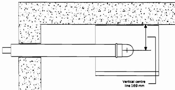
**10.4** When cutting the flue hole it is recommended that a 105mm diameter core drill is used where both internal and external access for the flue installation is available. Where only internal access is available a 125mm diameter core drill should be used. (NB. Please take adequate precautions to prevent debris entering boiler via flue connection).
