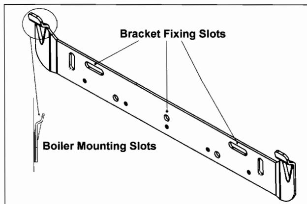
**10.6** Mount the boiler onto the fixing bracket via the boiler mounting slots. Ensure that the wall is capable to carry the boiler.
