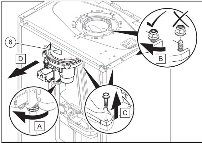
9. Remove the gas-air mixture unit (6).
