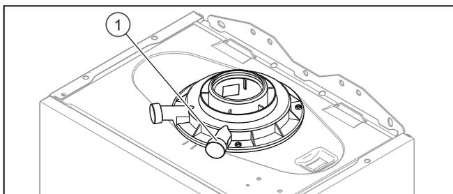
3. Unscrew the cover from the flue gas analysis point (1).
