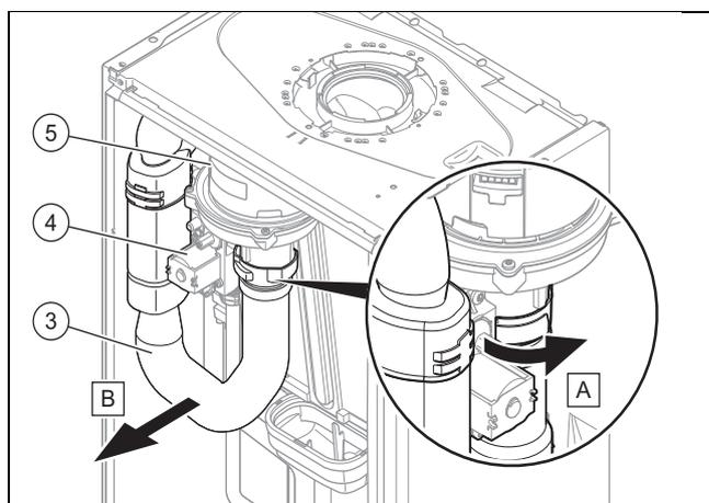
7. Remove the air intake pipe (3).
