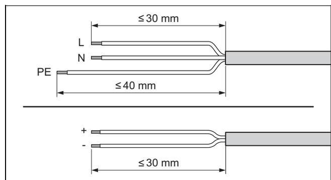
6. Strip the flexible cables as shown in the figure. In doing so, ensure that the insulation on the individual conductors is not damaged.
