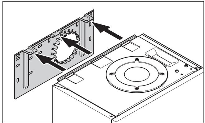
6. Mount the unit mounting bracket on the wall.
