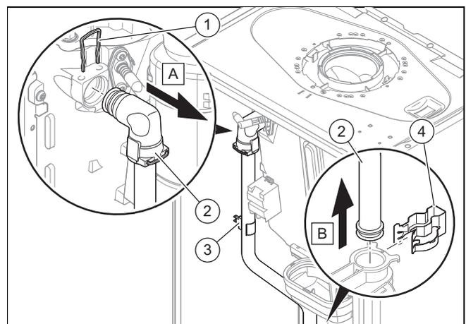
4. Remove the temperature sensor (3).
