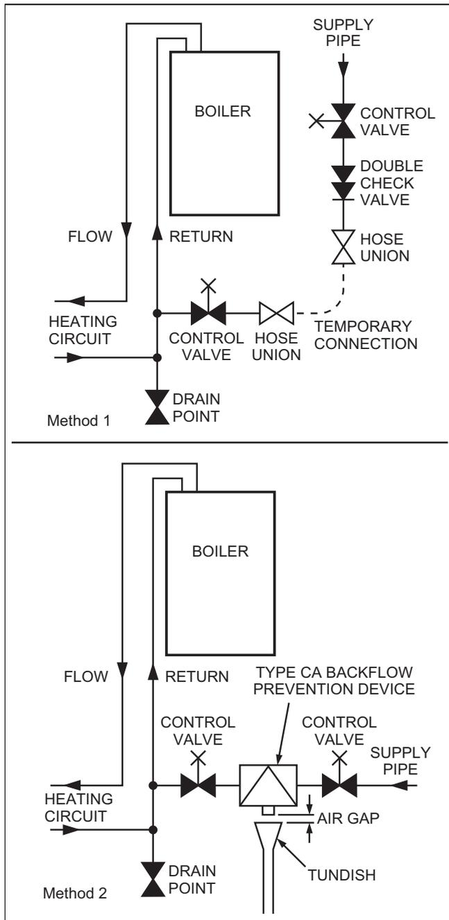
A safety valve must be fitted to a sealed system. It shall be preset, non-adjustable with a lift pressure of 3 bar, incorporating seating of a resilient material, a test device and a connection for drain. The drain from the safety valve must be routed outside the building, must not discharge above an en-
