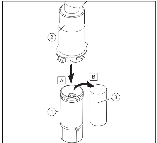
1. Unclip the lower section of the siphon (1) from the upper section of the siphon (2).
