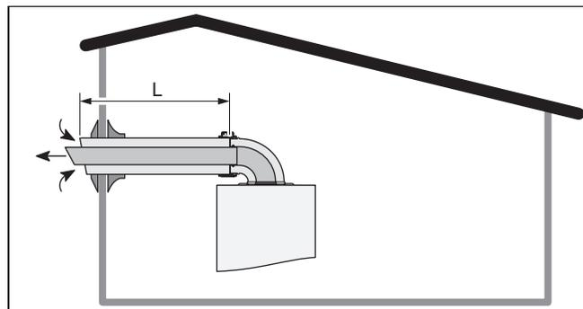
The openings in an attachment for separate lines must lead to a 50 cm-sided square.
