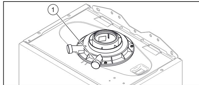
3. Unscrew the protective cover from the flue gas analysis point (1).
