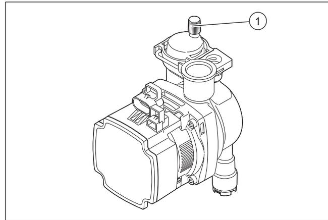
1. Loosen the purging valve cap (1) on the pump and on the automatic air vents.
