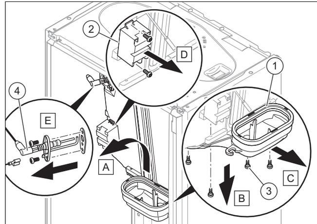
13. Lift the heat exchanger up slightly and remove it together with the condensate tray (1).
