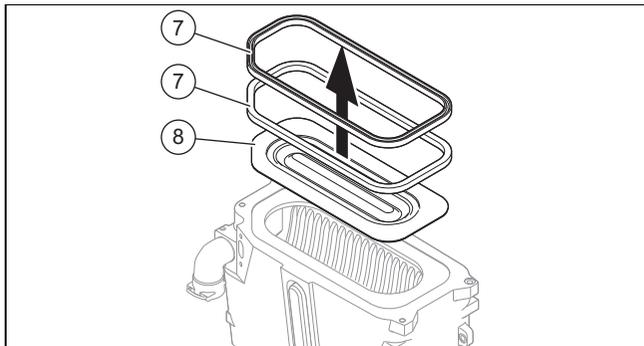
9. Remove the burner seals (7) and the burner (8).
