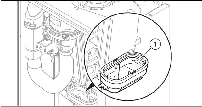
6. Using water to clean the condensate tray (1).
