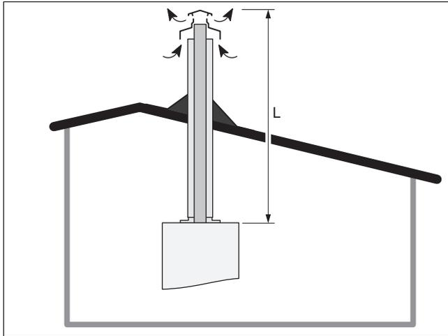
The openings in an attachment for separate lines must lead to a 50 cm-sided square.
