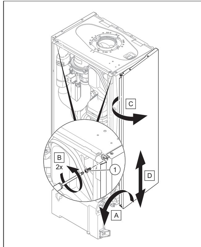
1. Tilt the electronics box forward.
