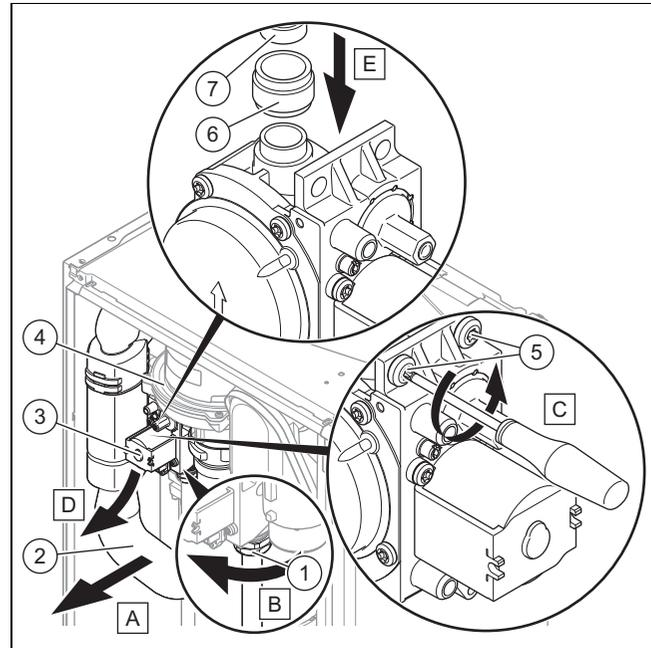
4. Remove the air intake pipe (2).
