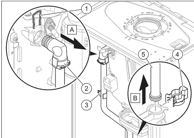
4. Remove the temperature sensor (3).
