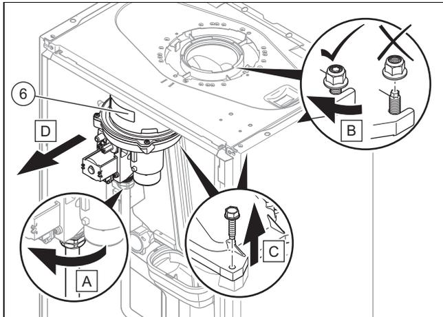
8. Remove the gas-air mixture unit (6).
