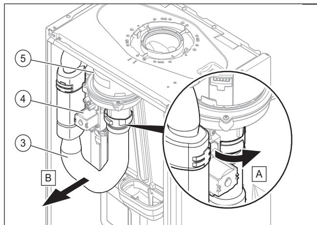
6. Remove the air intake pipe (3).
