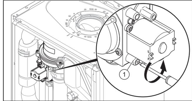
2. Use a screwdriver to undo the sealing screw on the measuring nipple (1) of the gas valve.
