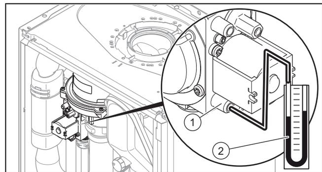
3. Connect a pressure gauge (2) to the measuring nipple (1).
