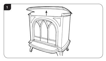
2.3 Lift the front upwards until it is clear of the slots and pull away from the appliance, see Diagram 2.
