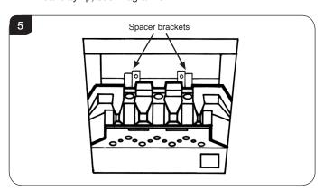
7.2 Locate the rear panel against the spacer brackets, see Diagram 5 and slide down so that it locates on the ledge of the flame baffle, see Diagram 6.
