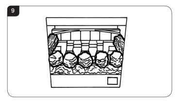
7.6 Place four of the loose round coals behind the first row so that they sit on the fingers of the flame baffle, the two outer ones should touch the rectangular coals, see Diagram 10.
