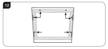
8.10 Replace ALL of the securing screws ensuring that a screw is present in all fixing slots.
