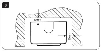
5.4 In a non-combustible recess be careful to allow enough clearance at the sides and rear of the appliance to perform spillage tests and reach the controls.
