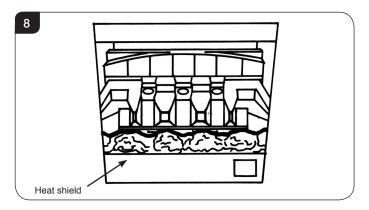
8.5 Place five of the loose round coals on the front coal so they lean against the flame baffle, in between the fingers. Place the two rectangular coals against the reflector panels, one either side, behind the front row of loose coals, see Diagram q
