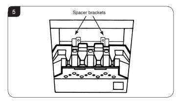
8.2 Locate the rear panel against the spacer brackets, see Diagram 5 and slide down so that it locates on the ledge of the flame baffle, see Diagram 6.
