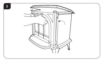
5.4 Remove the glass frame by undoing the fixing screws and lifting clear, see Diagram 4. Take care to support the glass window panel when removing the screws.
