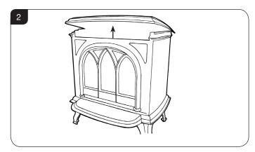
5.4 Lift the front upwards until it is clear of the slots and pull away from the appliance, see Diagram 3.
