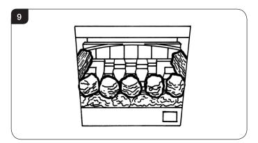
8.6 Place four of the loose round coals behind the first row so that they sit on the fingers of the flame baffle, the two outer ones should touch the rectangular coals, see Diagram 10.
