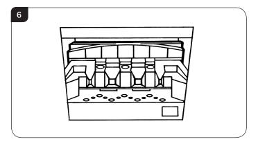
7.3 Place the coal retainer in the two guides as shown in Diagram 7.
