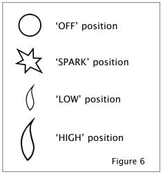
To achieve the HIGH setting, push the control knob in slightly and continue turning fully anti-clockwise to the high position. The main burner should light after a few seconds. To decrease the setting to LOW, turn the control knob clockwise to the low setting.
