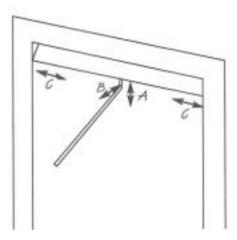
A.25mm down from top of opening B. 25mm in from front of opening.
