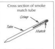
Take a length of 10mm dia pipe and seal one end. Crimp the pipe to prevent the match from sliding down inside
