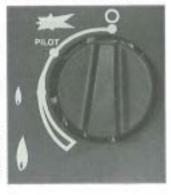
To turn to the PILOT position from the HIGH or LOW positions, press the control knob in, and return to the pilot position and release. To turn the fire OFF, keep the knob pressed in, return to the off position and release.
