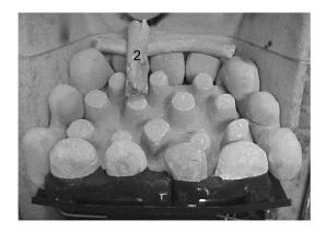
Place driftwood SHAPE No. 3 in position as shown. The recess in the base should locate over the RH Front Matrix and the arrow, marked on the base, should point towards the rear of the appliance.
