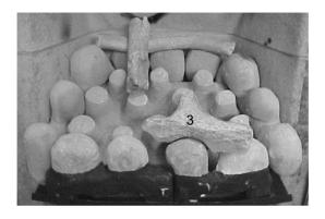
Place driftwood SHAPE No. 4 in position as shown. The arrow, marked on the base, should point towards the rear of the appliance.
