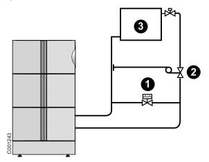
Poor adjustment of the differential valve may cause a continuous increase in the return of water to the boiler.
