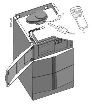
► Run the boiler at full-load by pressing "♦" and [+]-keys simultaneously.
