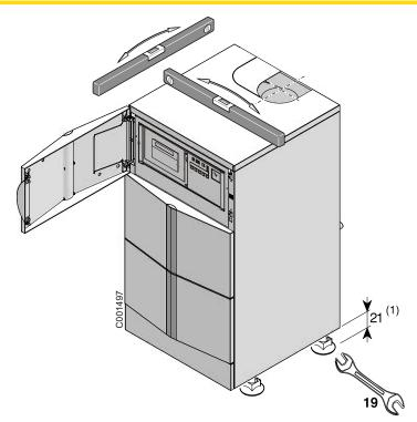
Level the boiler by turning the adjustable feet. To adjust, take the load off the foot using a lever.
