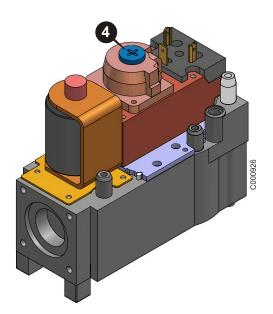
If the values exceed the tolerances: Check the gas input pressure. Check that the restrictor fitted is suitable for the gas being used (G20 = diameter 8.6, Propane = 6.7).
