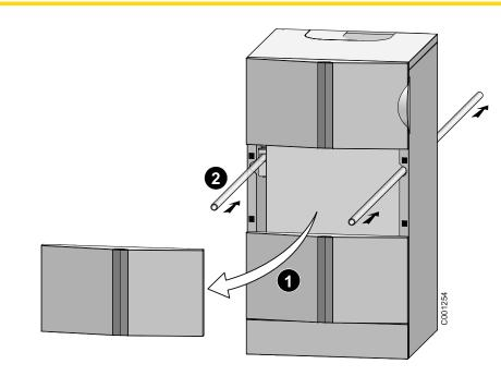
**1** The boiler can be lifted by using 2 tubes Ø3/4" placed as shown in the view.
