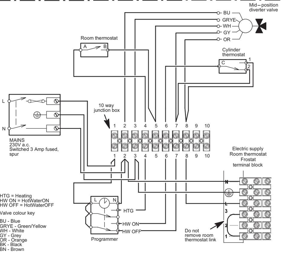
Fig. 6.29 - Not permanent live Y - plan
