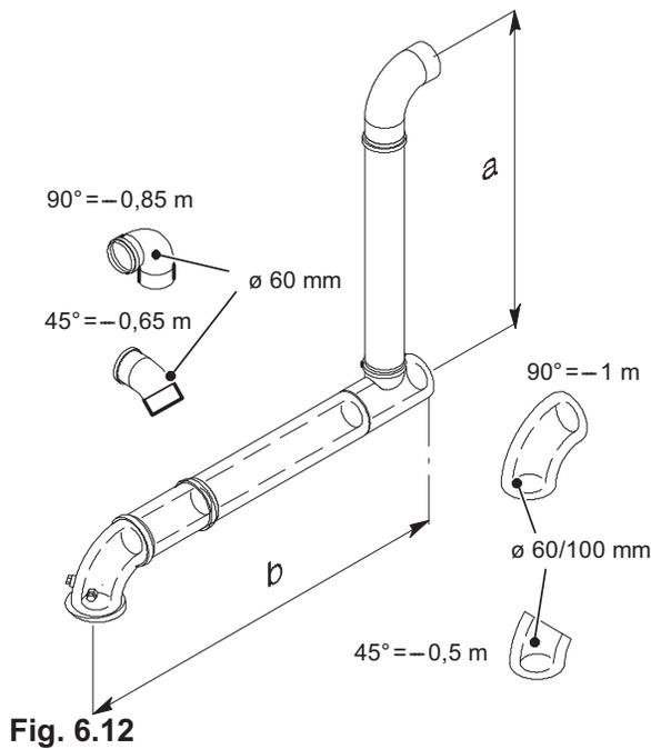
In the last section, the fumes are expelled through a vertical section.
