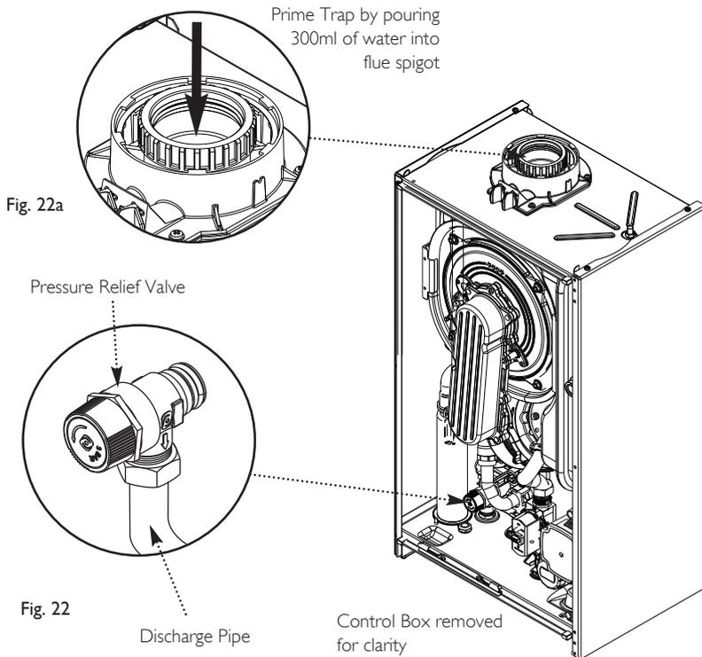
1. Remove the discharge pipe from the kit.
