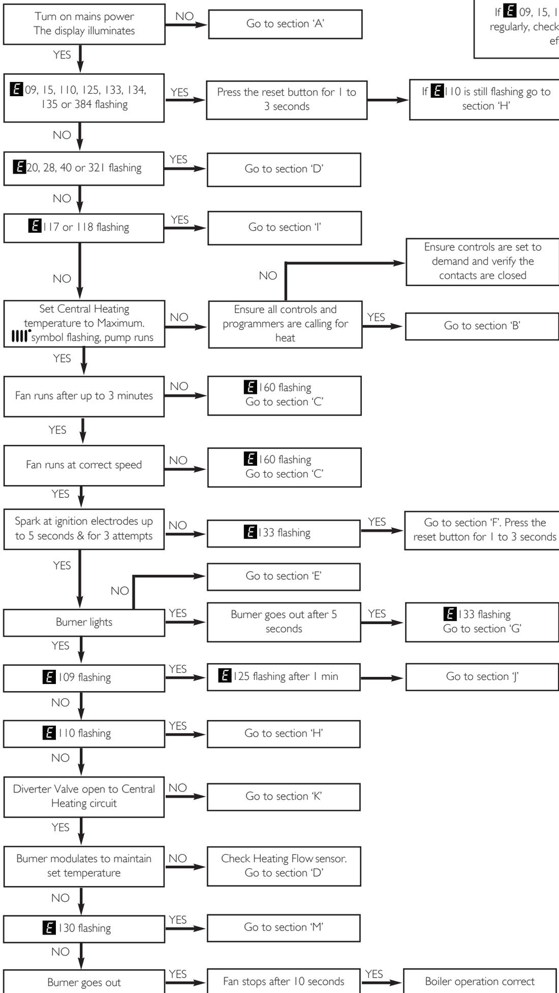
If **E 09, 15, 110 or 384** is flashing or re-occurs regularly, check all PCB connections. If this has no effect replace the PCB.
