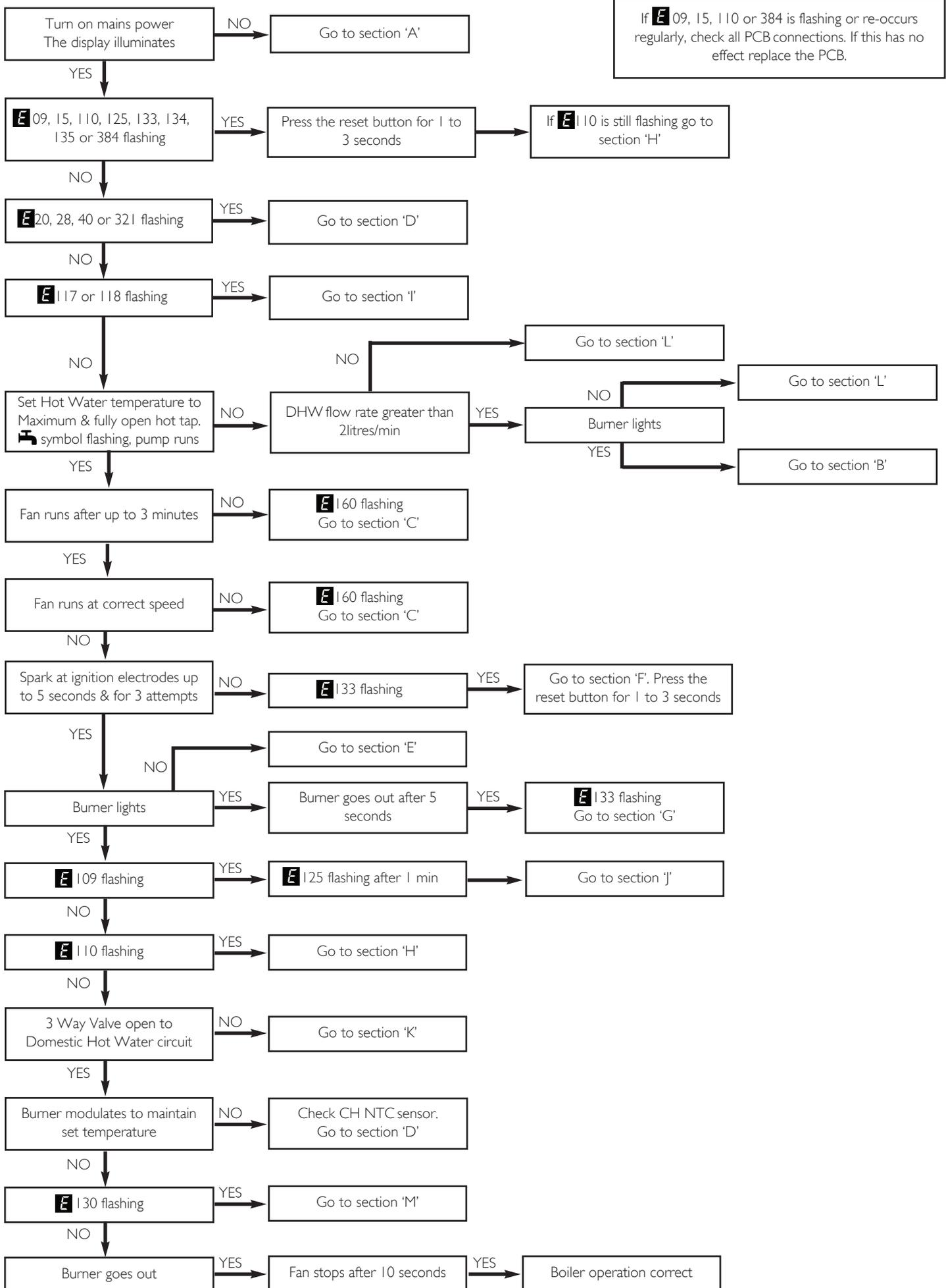
If E 09, 15, 110 or 384 is flashing or re-occurs regularly, check all PCB connections. If this has no effect replace the PCB.
