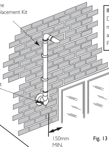
**IMPORTANT:** If fitting a Plume Displacement Flue Kit, the air inlet must be a minimum of 150mm from any opening windows or doors (see Fig. 13).
