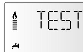
Rotate the encoder
