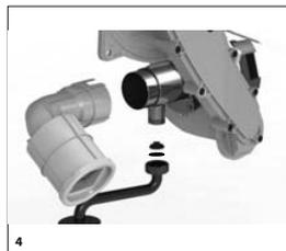
7. Reassemble the gas supply onto the venture assembly (fig 4)
