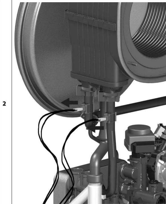
Remove the clip and the temperature sensor
