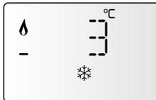
If the central heating flow temperature is < 3°C, the burner will fire (heating position) at minimum power until the temperature reaches > 30°C, the burner will go out.
