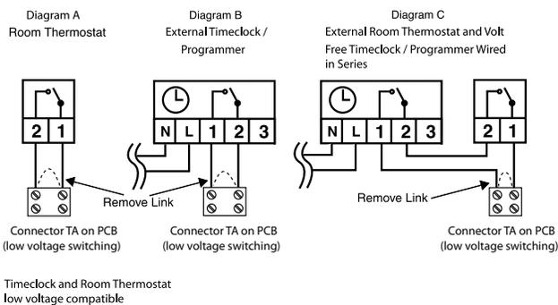
DO NOT CONNECT 240V TO ANY PERIPHERAL CONNECTIONS
