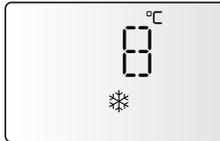
If the flow temperature remains between 3°C and 8°C the pump will continue to run for a maximum of 20 minutes unless a temperature above > 9°C is detected in the central heating flow, after this the burner will fire (heating position) until a temperature of > 30°C is detected.
