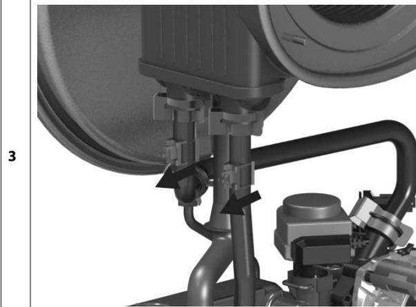
**IMPORTANT !** Do not use conducting paste for the contact sensors because it will alter the resistance value.
