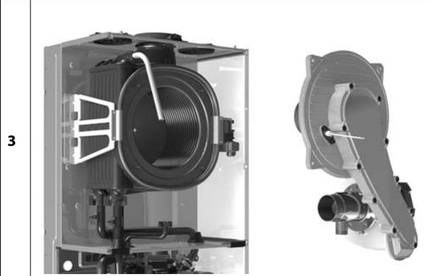
Remove the ten screws to free the burner door
