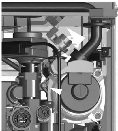
Disconnect the pipe and then move the pump to the right to disengage
