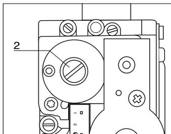
**Attention!** If the value of the CO<sub>2</sub> at the minum power has been changed, it is necessary repet the adjusting at maximum gas flow.
