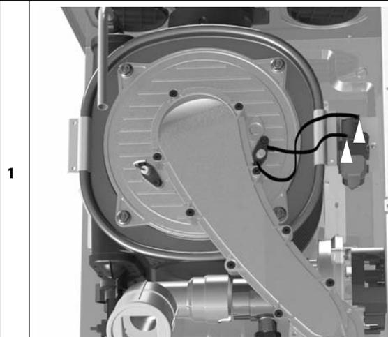
Remove the screws and the spark generator
