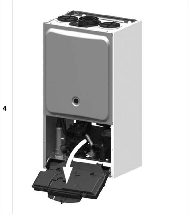
Remove the combustion chamber front panel by releasing the clips
