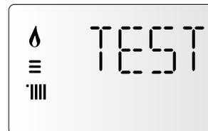
On the display appear TEST and the icon
