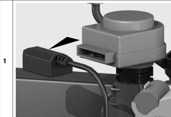
Remove the clip and lift the motor from the diverter valve body.
