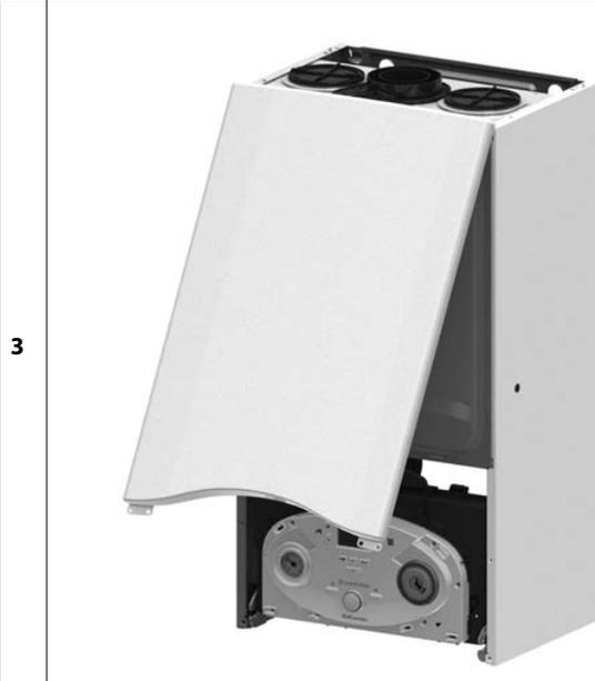
Lower the electrical front panel
