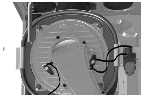
Remove the screws and pull the electrodes towards you.
