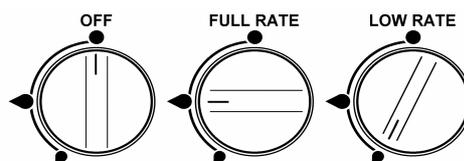
To light the burner, press in and turn the knob anti-clockwise to the full rate position and apply a light to the burner or press the ignition button if fitted. It is necessary to hold the knob depressed during ignition and for approximately fifteen seconds after the burner has lit to allow the probe to
