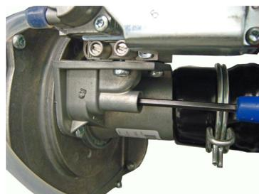
9. Follow the commissioning procedure in section 5.2.2 (points 1 to 36) from page 43 with the exception that the **The CO<sup>2</sup> combustion figure should now be 10.2% +/- 0.2% for LPG**
