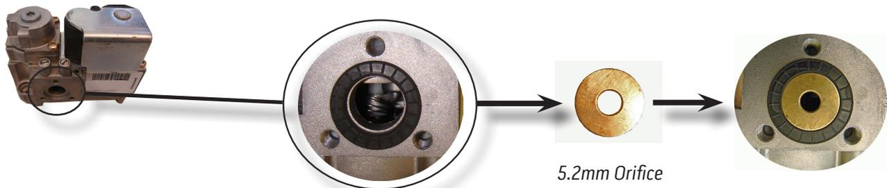
5. Re-secure the gas valve to the venturi.
