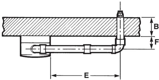
$L = B + E + F + 245 \text{ mm} + (90^\circ \text{ bend} = 1.3 \text{ metre})$
