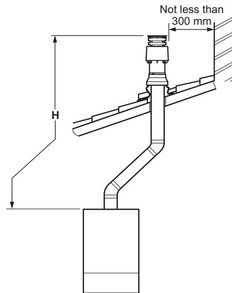
$H_{\text{max}} = 12.2 \text{ m } (14 \text{ m} - 1.8 \text{ m})$
