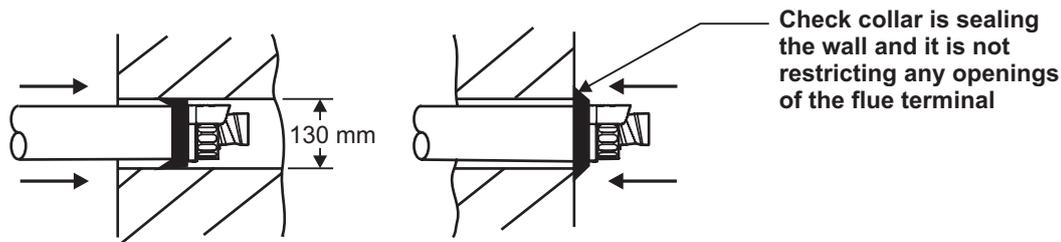
**Fig. 5.8 - Fitting the flue from inside**
