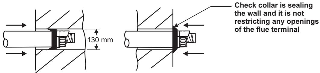
**Fig. 4.8 - Fitting the flue from inside**
