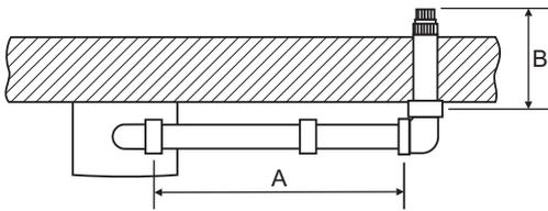
$L = A + B + (90^\circ \text{ bend} = 1.3 \text{ metre})$
