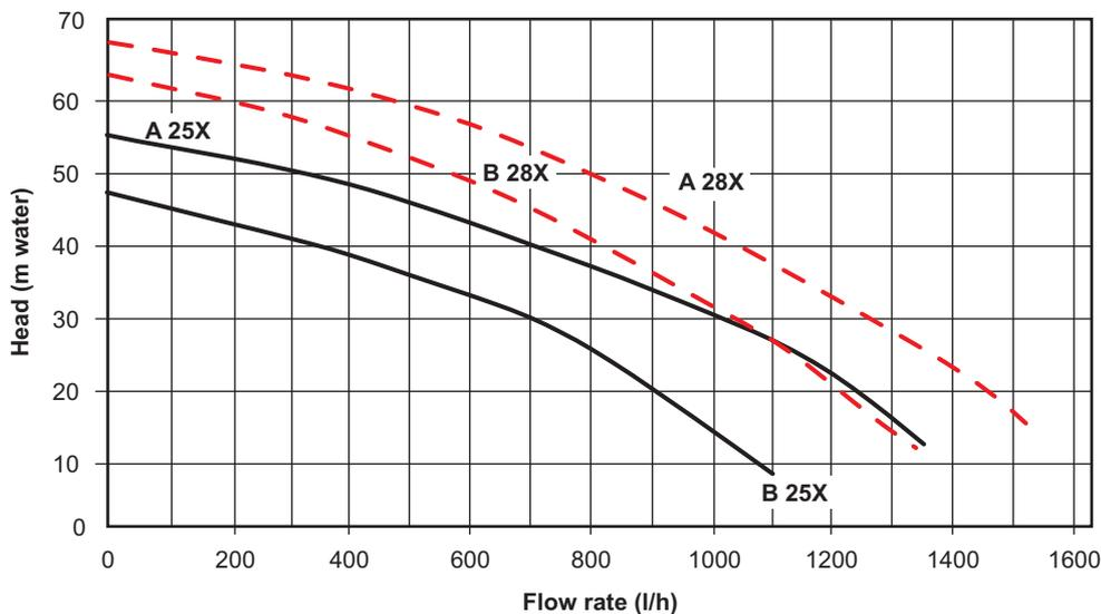
A = Head available to the system at pump speed 3 (by-pass closed)
