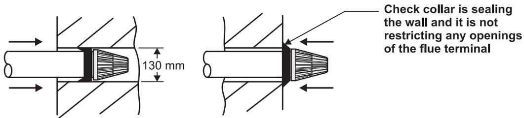
**Fig. 17 - Fitting the flue from inside**
