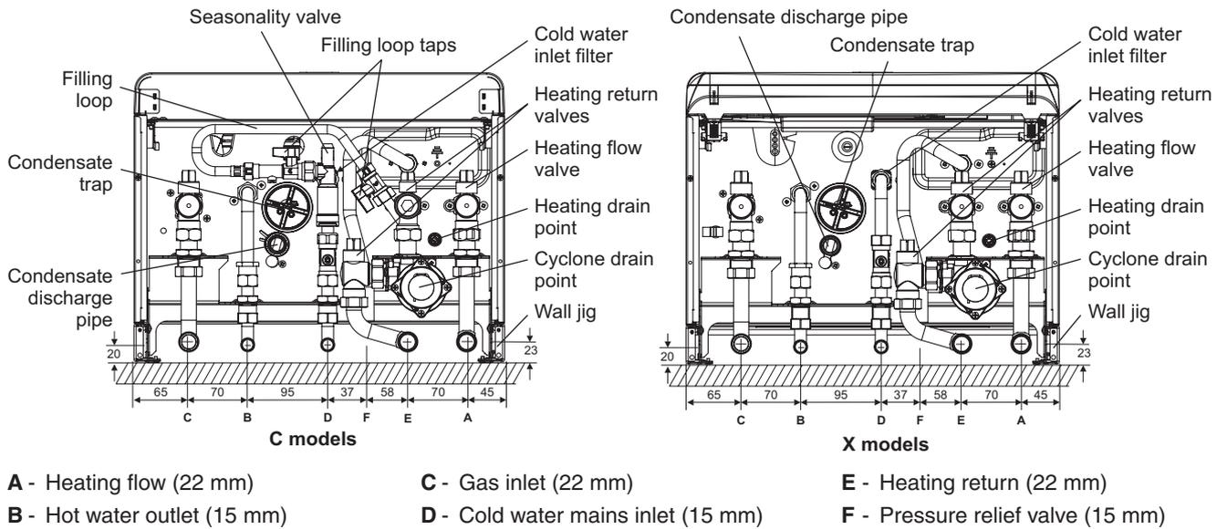
Fig. 13b - With wall jig
